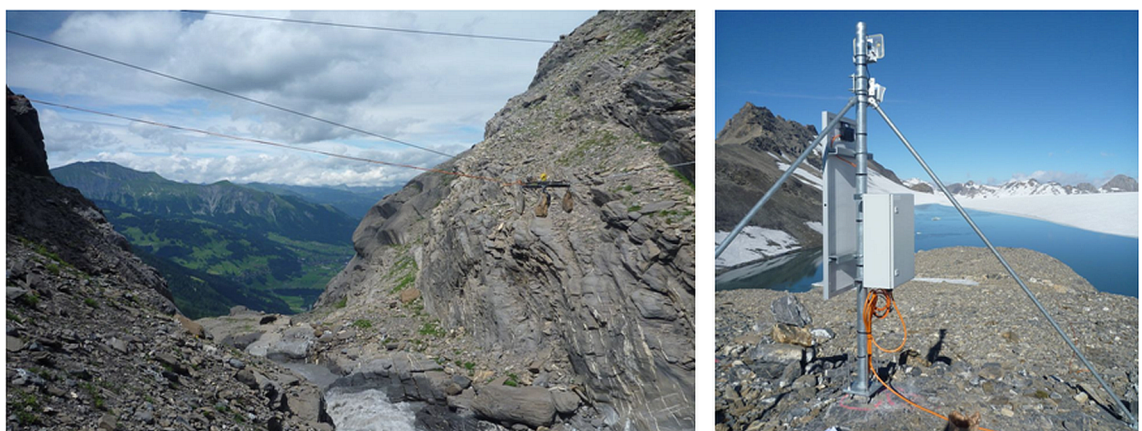
FIGURE 2.21: Sensors of the Plaine Morte Warning System: a radar detects floods in the catchment (left), pressure sensors monitor the lake levels (right), (GEOPRAEVENT AG, 2015).
