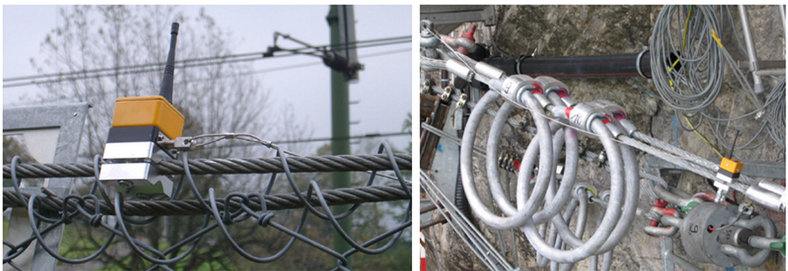
FIGURE 2.23: Sensors of the SBB Alarm System: seismic sensors detect ground shaking (left), tripwires are pulled-out when nets are hit by rocks (right), (SBB, 2011).
