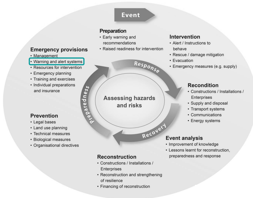
FIGURE 1.2: Cycle of Integrated Risk Management: includes mitigation measures to reduce the risk imposed by natural hazards to an acceptable level (FOCP, 2012).
