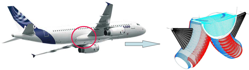
Figure 1.2: Bulkhead location. Source [EAD].
