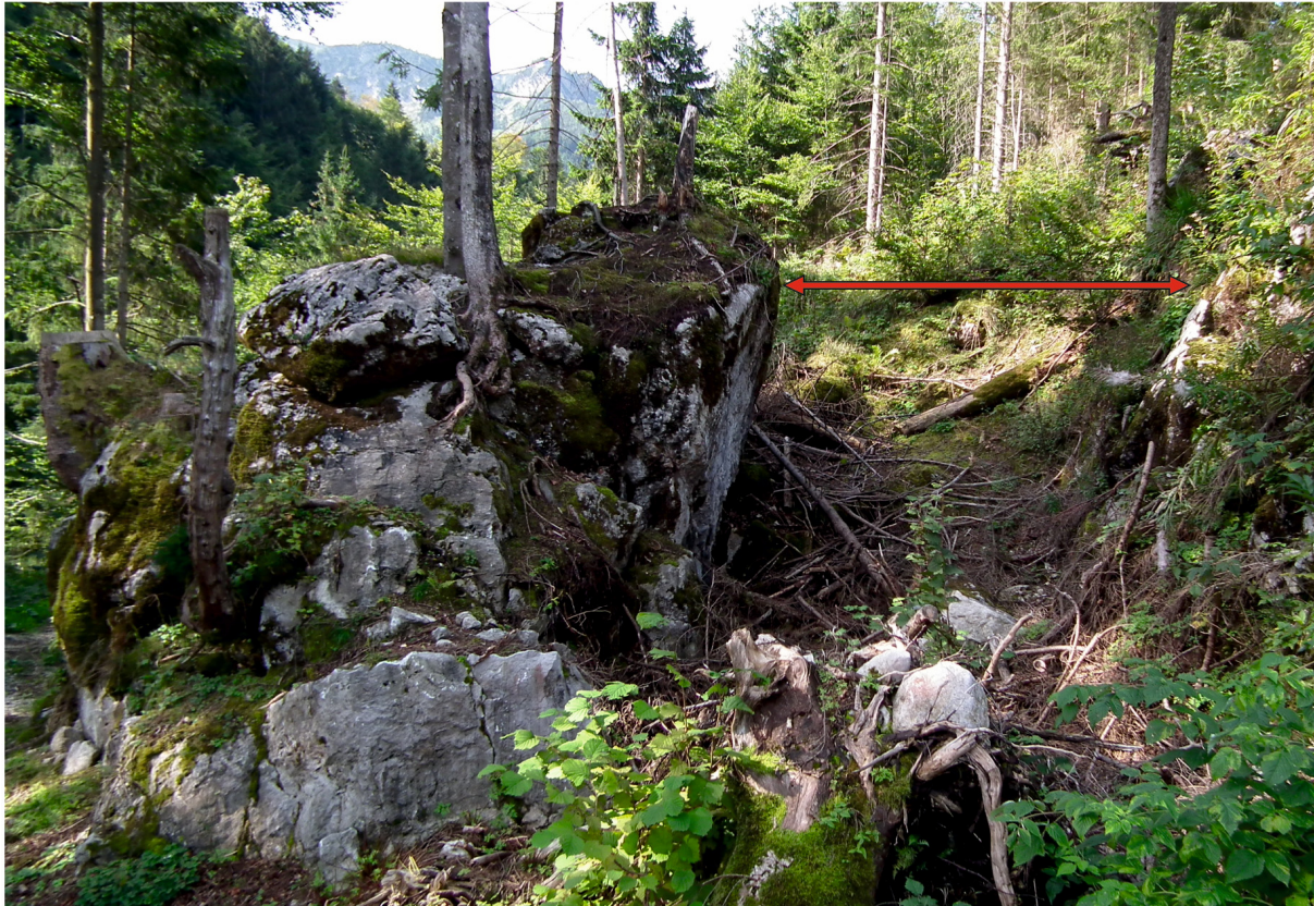
Figure 20: Tension crack within an Upper Rhaetian limestone block at the back of the landslide's over-steepened front. The crack's opening width is about 4 m, accentuated by the red arrow.
