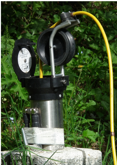
Figure 34: Top of the inclinometric measurement site at KB1. The yellow measurement cable is connected to the probe (in the casing – not pictured) and can be pulled up and be clamped in the jaws of the pulley at the 0.5 m intervals. On the left, outside of the casing, the connectors of the TDR system installed parallel to the inclinometer are visible.
