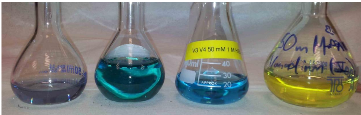
Figure 5.5 - Photograph of 0.1 M vanadium species in 1 M H_2SO_4 prepared for this study. From left to right: V^{2+} (purple), V^{3+} (green), VO^{2+} (blue) and VO_2^+ (yellow).
