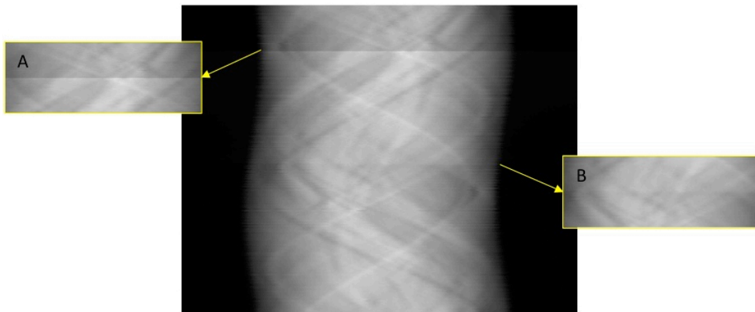
Figure 5.8: The illustration of the tube current drop. In this acquisition, there is a change in intensity as shown in box A, due to the drop in tube current. This lasted for several projections before the condition normalized again, as can be seen in B
