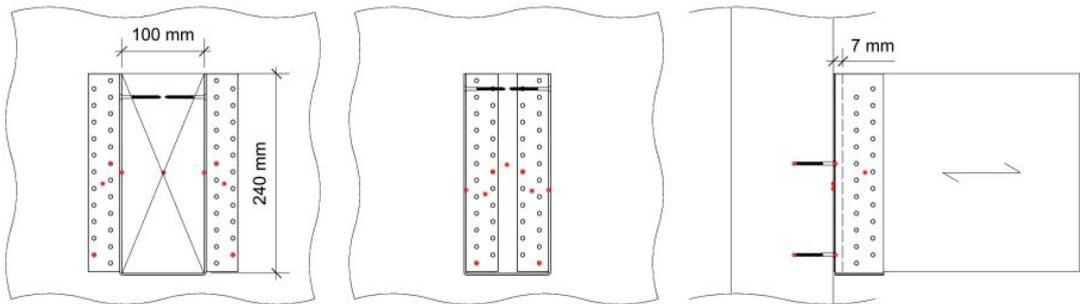
Figure 3. Exemplary fire test setup for joist hangers.
