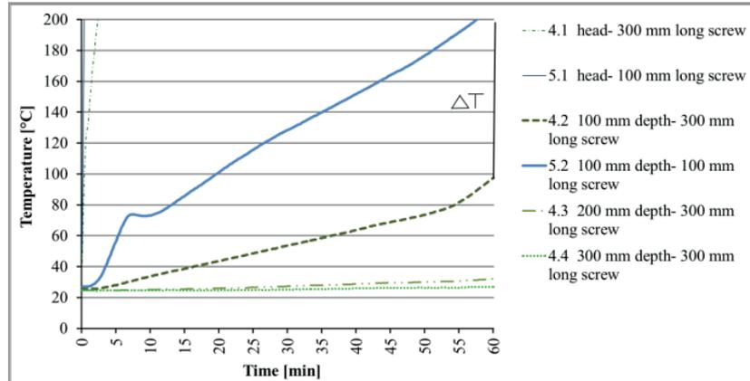
Figure 6. Temperature development for two counter sunk head full thread screws  $\text{Ø}_n$  8 mm.
