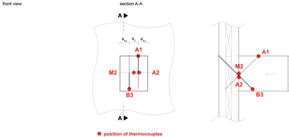
Figure 5. Crossed screws and position of thermocouples in the connection (schematic illustration).
