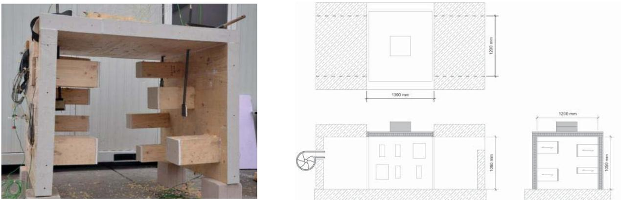
Figure 2. Left: assembled specimen with measurement equipment, right: drawing of furnace and specimen.
