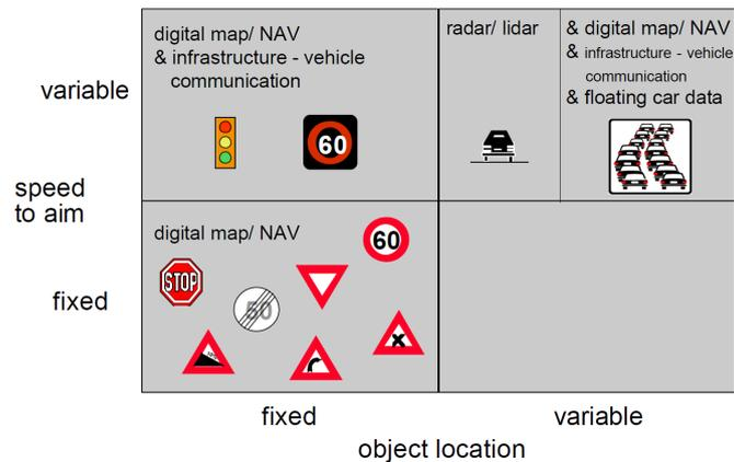
Figure 3.2.: Classification for deceleration situations with two dimensions: speed to aim (variable & fixed) and object location (fixed & variable) by Reichert et al. [142]
