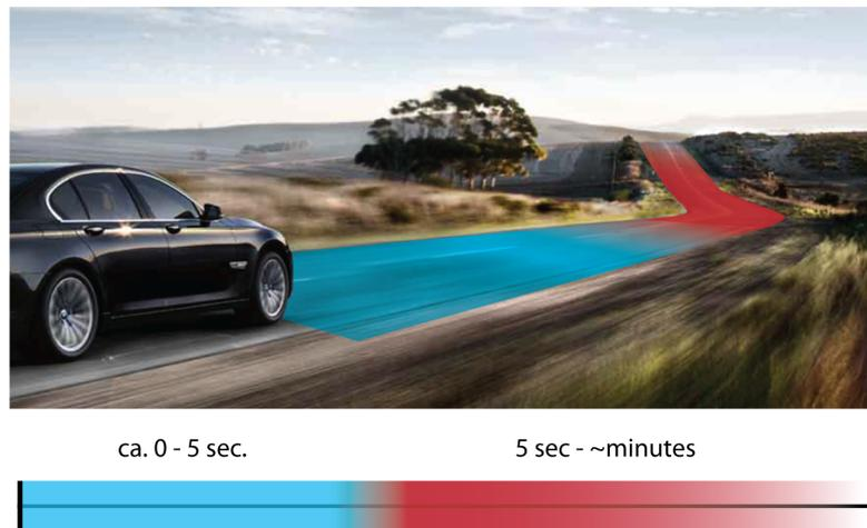
Figure 2.1.: Schematic view on the currently available information sources (blue) and the enlarging of this horizon to an electronic horizon with the help of new information sources (red) like digital maps or the Car2X infrastructure
