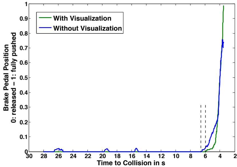
Figure 8.9.: “Complete Miss”, comparison of the brake pedal position over TTC
