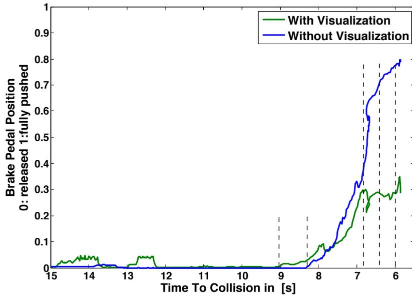
Figure 8.5.: “Partial Miss” situation, comparison of the brake pedal position over the TTC
