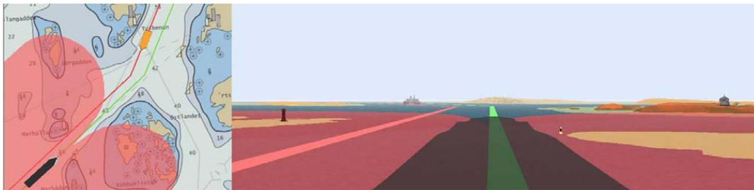
Figure 4.4.: Real-time 3D nautical chart: Red areas or non-reachable, the trumpet in front of the vessel indicates the maximum turning angle, from Proathe [136]
