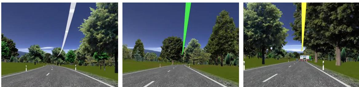
(a) Idle state, no request for action, solid white line (b) Deceleration situation, request for action: "release gas", solid green line (c) Deceleration situation, request for action: "step on brake", solid yellow line
