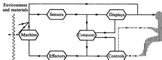
Figure 7.1.: The control loop with computer assistance: operator can use the controls in order to alter the machine state and can control his actions via a display output. Controls and display output are supported by a computer, from Singleton [160]
