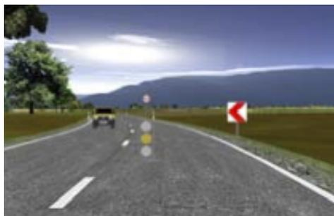
(a) Warning variant realized inside driving simulator environment, a traffic light metaphor indicates the driver to adjust the speed
