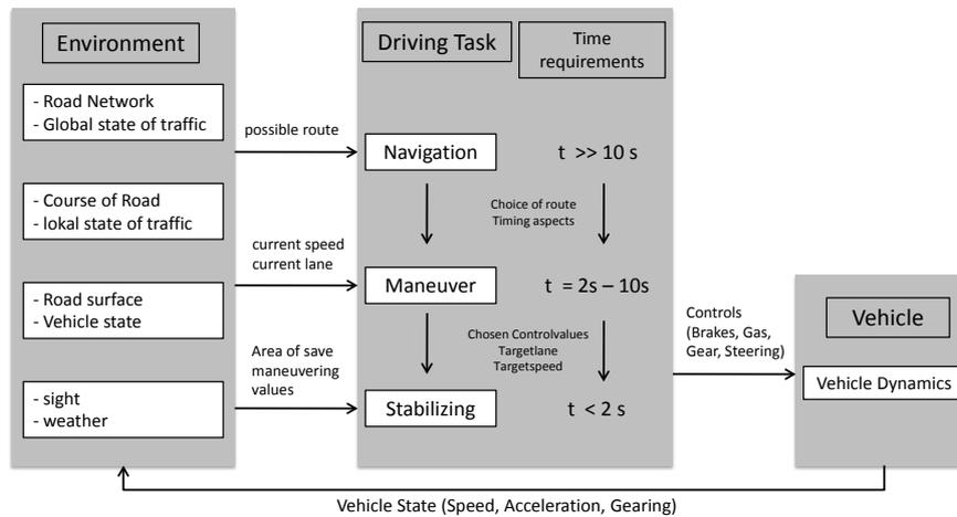
Figure 2.8.: The three layer model distributed over the environment, the driving task and the vehicle; Including timing aspects; after Bernotat [19] from Deutschl [50]
