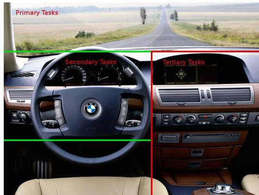
Figure 2.7.: Distribution of the primary (out the window), secondary (steering wheel & IC) and tertiary task (center dash) in a 7 series BMW, from Toennis et al. [173]
