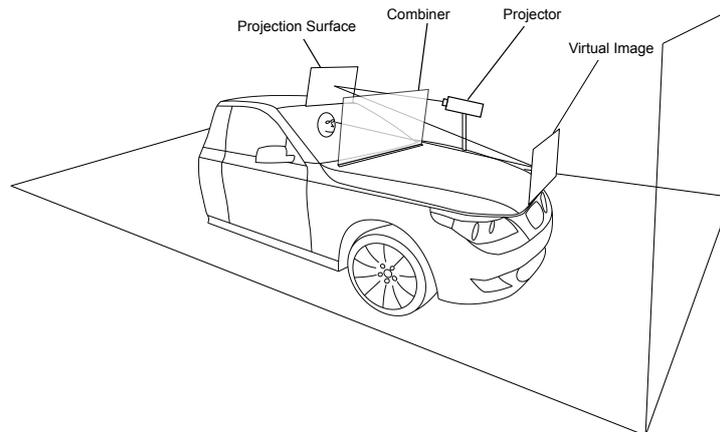
Figure 5.2.: Driving simulator mock-up for the video experiment including the custom HUD construction
