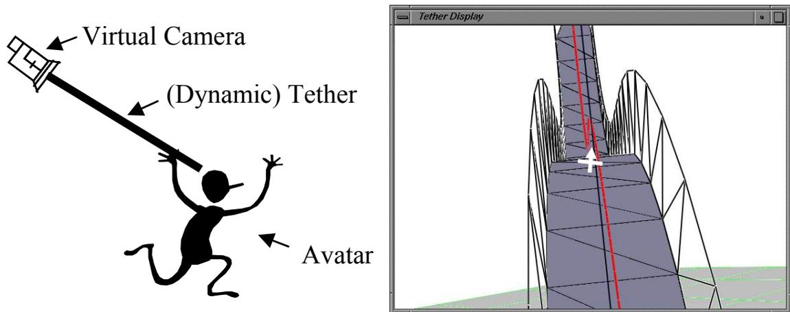
(a) The dynamically tethered virtual camera observing an avatar from an ego referenced POV (b) Navigation task through a virtual tunnel with a small white plane that is observed by tethered POV
