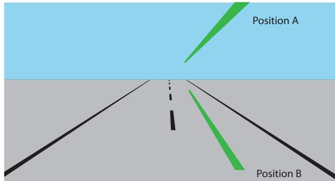
Figure 4.29.: Possible positions of the VRL (green), directly on the street (Position B) or above the head of the observer (Position A)
