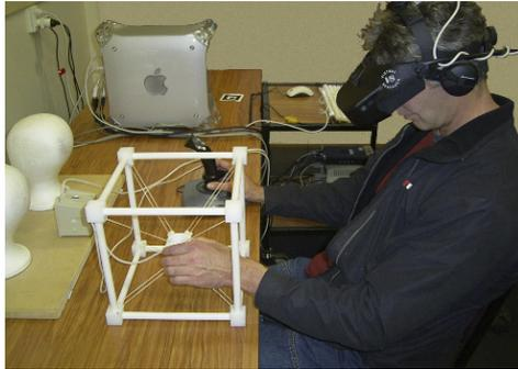
(a) Setup for experiment, the uses a HMD and two joysticks in order to control the SRMS
