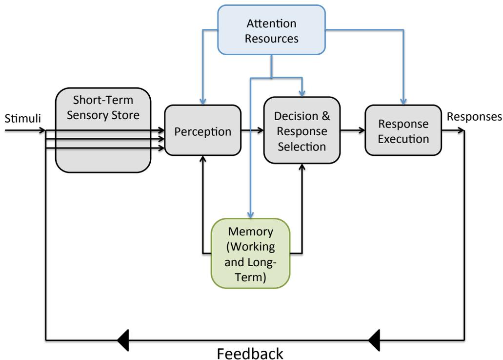
Figure 2.4.: Information processing model: a stimulus is received via the human sensors, it is perceived, a decision is made, a response is executed and finally a feedback is given; adapted from Wickens & Hollands [195]
