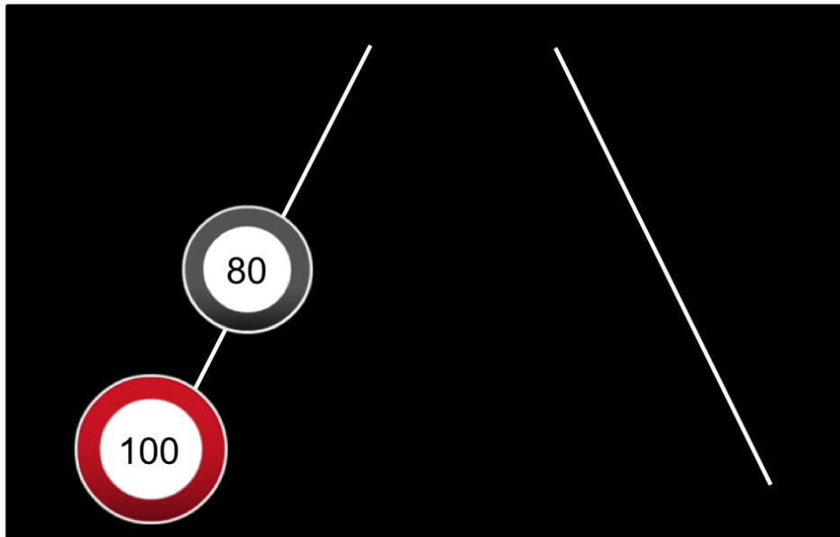
Figure 10.2.: Abstract visualization of the user Interface of the deceleration assisting system, lower left corner: currently valid speed limit sign (ref border); above: next speed limit sign (gray border); signs are on piece of virtual street
