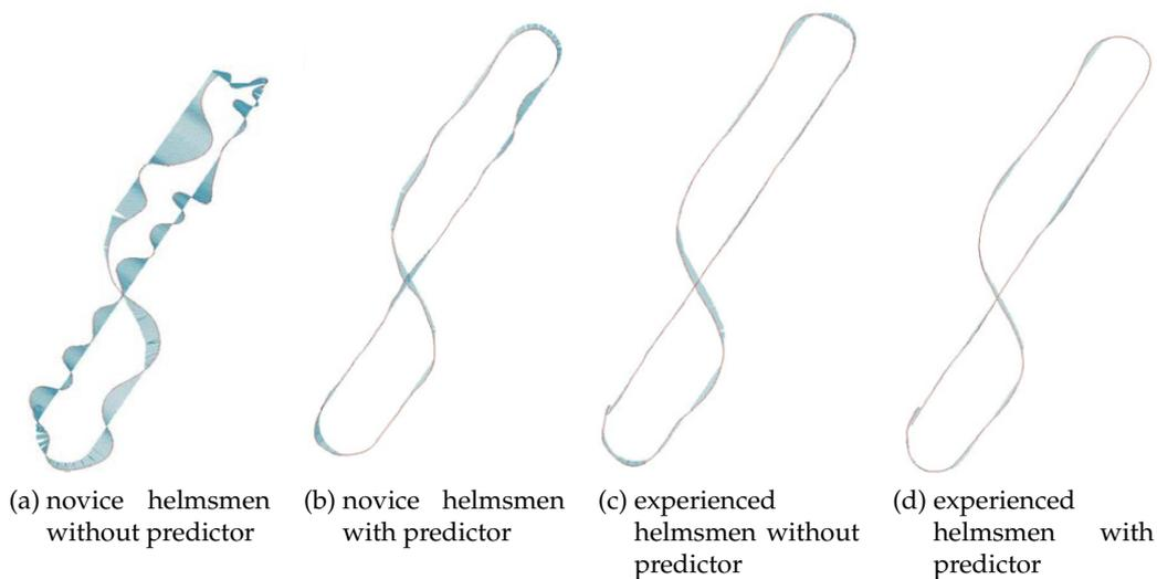
Figure 4.3.: Cross track distance for a figure 8 course, comparison between novice and experienced helmsmen, with and without predictor display, from Sullivan et al. [168]
