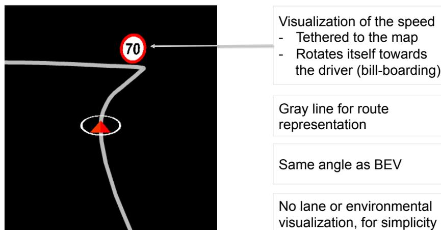
Figure 4.25.: Details of navigational view of the Navimap, simple situations are presented in this view
