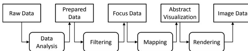
Figure 9.3.: The visualization pipeline, raw data enters the pipeline and with the help of four transformations image data is produced, adapted from Santos & Brodlie [148]
