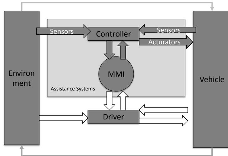
Figure 2.10.: Control Circuit ADAS: displaying the function and interaction of an ADAS between the environment, the MMI, the driver and the vehicle; from Deutschl [50]
