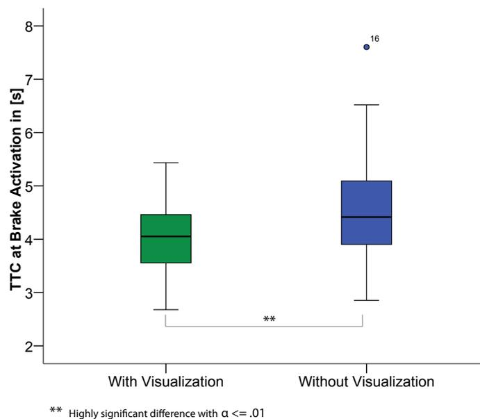
Figure 8.10.: “Complete Miss” situation, comparison of the TTC at brake activation
