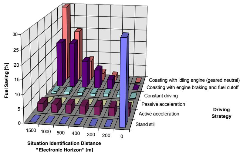
Figure 2.3.: Potential of different situations; The higher the distance the identification distance, the higher to potential energy saving potential, especially while coasting; from Reichert et al. [142]
