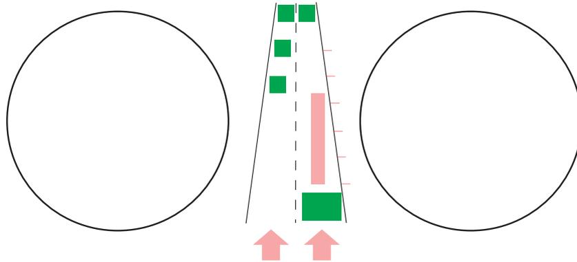
Figure 4.12.: Abstract visualization of the BEV in the instrument cluster, green elements were realized, red elements were discarded
