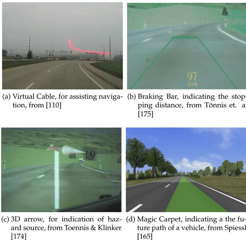
Figure 4.27.: Related work: contact analogue automotive visualizations from different
