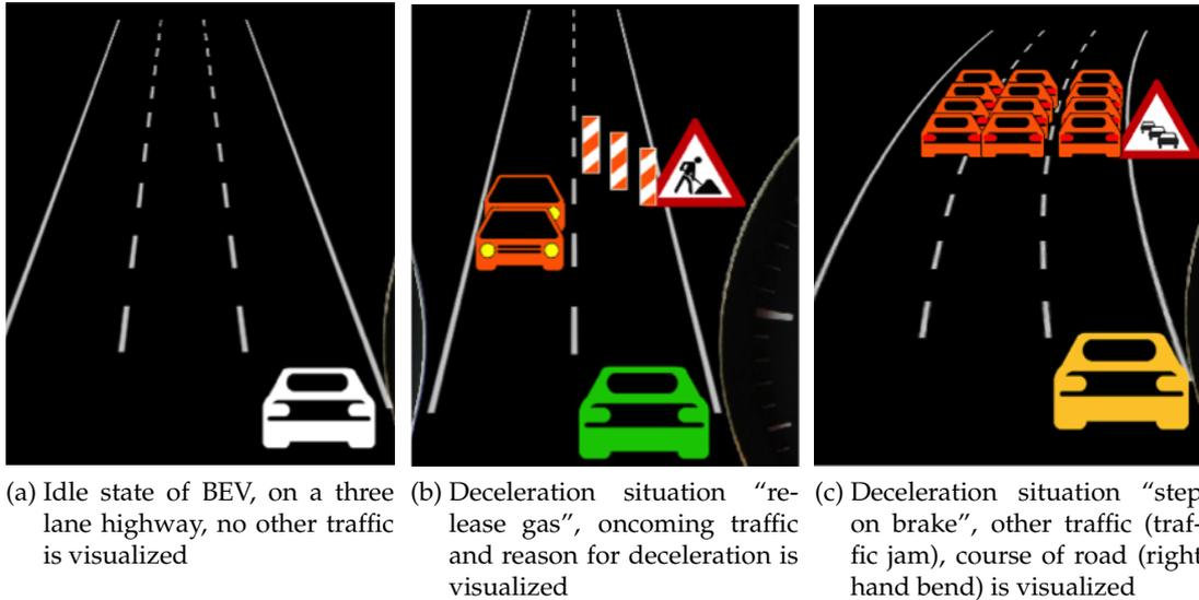
Figure 4.18.: Map details visualized in the idle state of the BEV and in deceleration situations
