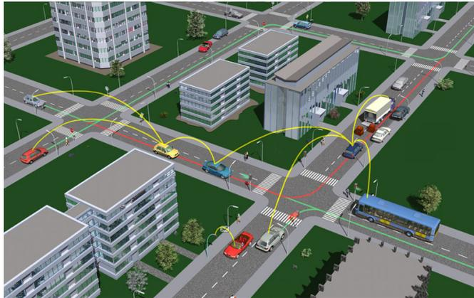
Figure 2.2.: Car2X-Communication Scenario, communication between vehicle, public transport and infrastructure; Baldessari et al. [12]
