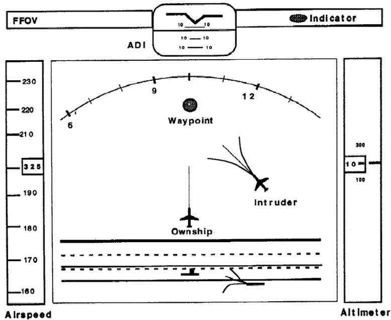
Figure 4.5.: Wegde Predictor Display: Shows “ownship” position with predicted path, as well as the intruder’s most likely path visualized by a wedge, from Gempler et al. [75]
