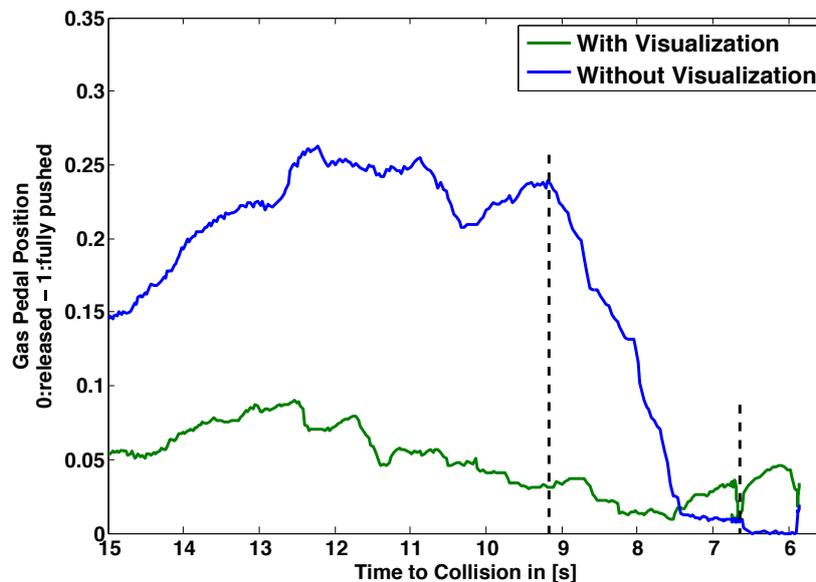
Figure 8.4.: “Partial Miss” situation, comparison of the gas pedal position over TTC
