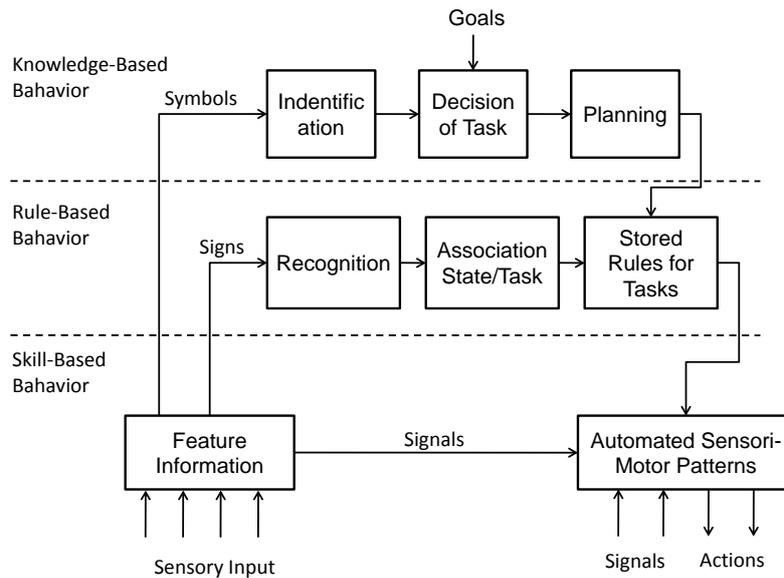
Figure 2.9.: Three levels of behavior; After a sensory input, action can either be skill-based, rule-based or knowledge-based, with differing amount of cognitive effort; after Rasmussen [140]
