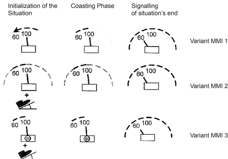
Figure 3.3.: Three MMI variants for assisting the driver in early deceleration. Indication in the speedometer and two variants with the support of an active gas pedal, by Samper & Kuhn [147]
