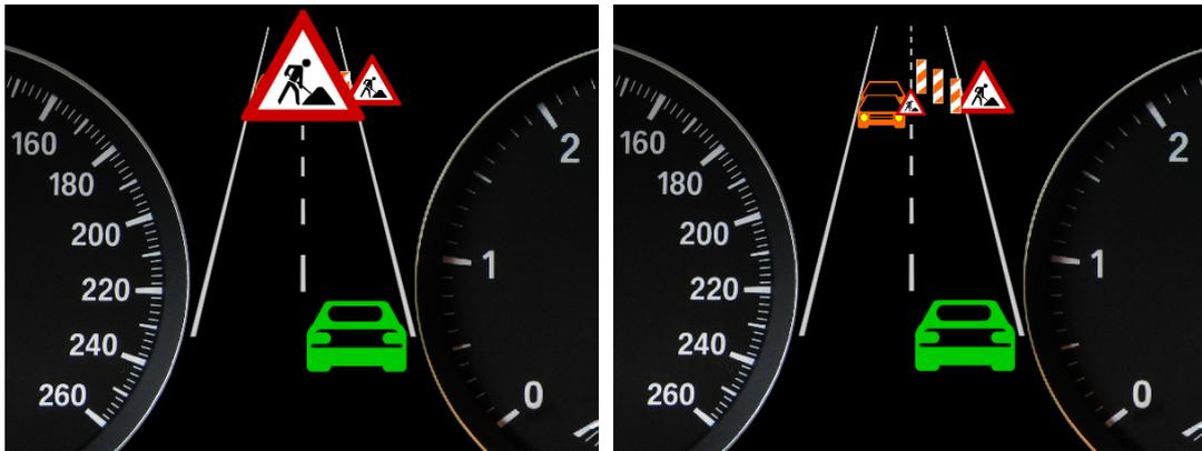
(a) Big traffic sign popping-up when the situation is recognized, sign represents situation (b) With the use an animation the sign gets smaller and fades out
