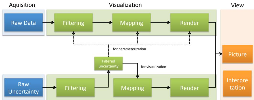
Figure 9.4.: The Visualization Pipeline including uncertainty: uncertainty can either be used to parameterize the raw data or it can be used for an additional visualization, adapted from Boukhelifa [24] and Griethe & Schuhmann[79]
