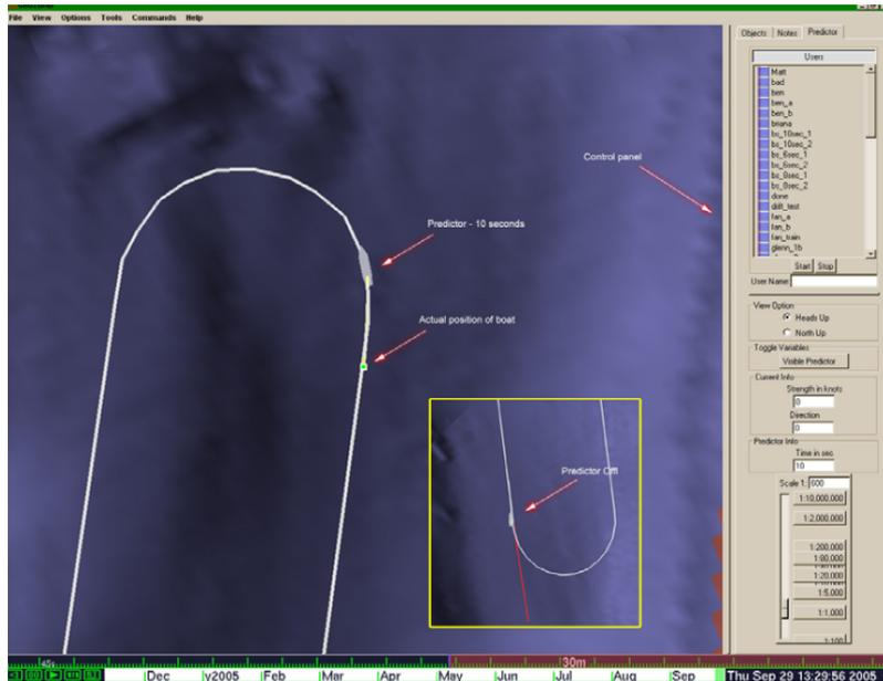
Figure 4.2.: Predictive Display: showing actual position and predicted position in ten seconds time, from Sullivan et al. [168]
