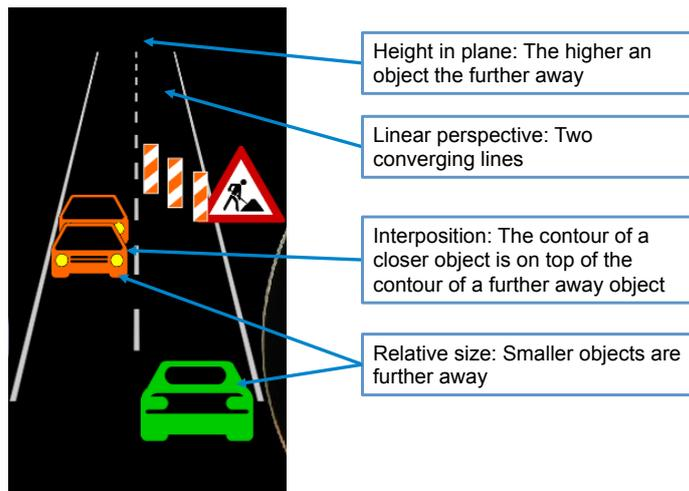
Figure 4.15.: Object oriented depth cues realized in the BEV in order to realize a 3D visualization on a 2D screen
