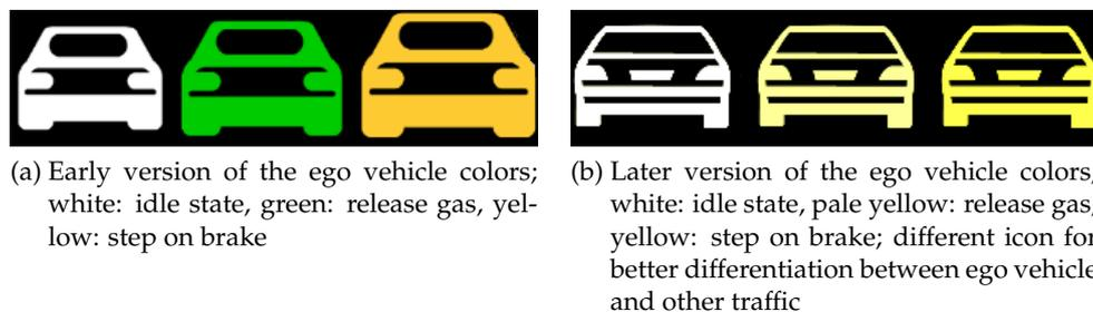
Figure 4.17.: Change in colors and icon of the ego vehicle in the BEV between the second and third evaluation
