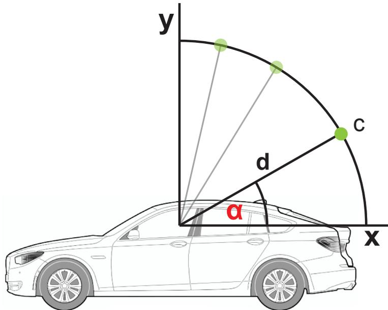
Figure 4.13.: The possible points where the POV can be located on a quadrant around the driver's head,  $\alpha$ : the rotation around the x-axis, d: the radius of the quadrant and the distance from the virtual vehicle to the virtual camera (c = location of virtual camera)
