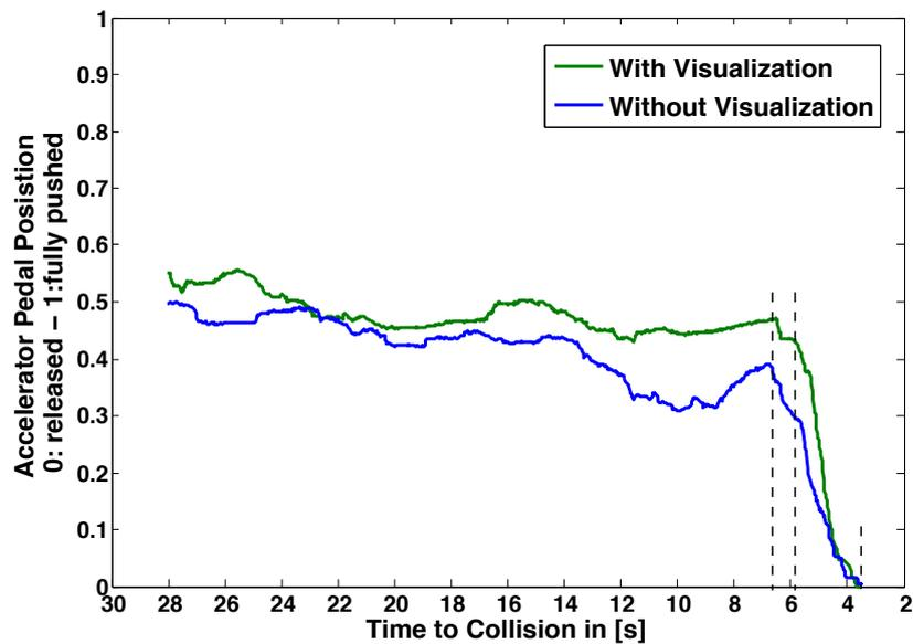
Figure 8.8.: “Complete Miss”, comparison of the gas pedal position over TTC
