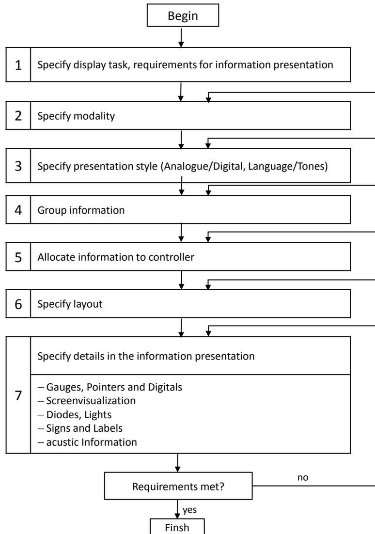
Figure 4.1.: The process of creating an automotive user interface in seven stages, from defining the requirements to implementing specific details; by Kirchner & Baum [94]
