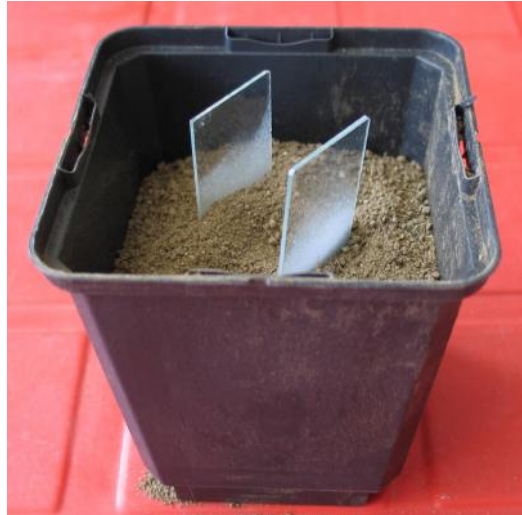
Figure 2.2 Image of the artificial rhizosphere model (ARM). The ARM consists of glass slides covered with an artificial exudate/agarose mix incubated in soil.
