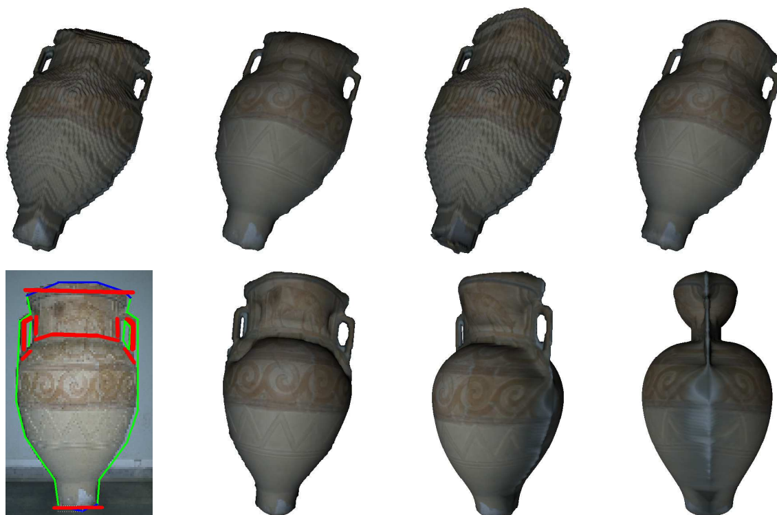
Figure 6.5.: Top row: shape priors and corresponding reconstructions with and without marked sharp contour edges. Bottom row: input image with marked contour edges (blue) and line strokes (red) for local discontinuities which are shown right.
