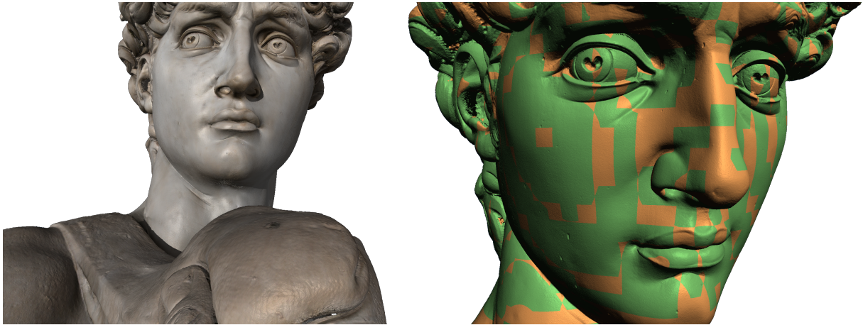
Figure 7.1: A 1 billion triangle model is rendered on a 1920 \times 1080 viewport using rasterization and ray-casting simultaneously. Ray-casting works on a sample-based surface LoD representation at an effective maximum sampling resolution of 8K^2 \times 32K . Red and green surface areas indicate parts of the model that are rendered via rasterization and ray-casting, respectively. On a GTX 680 graphics card the hybrid approach always renders the model in less than 30 ms ( > 33 fps) at a screen space error below pixel size.
