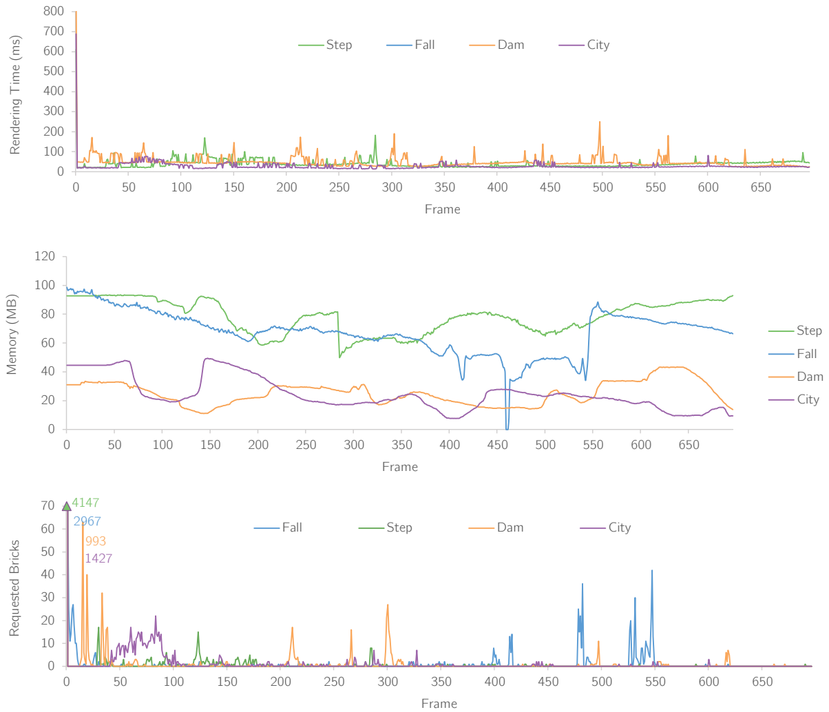
Figure 6.17: System behavior during data exploration of a single time step with different views and zooms. Note that the graph for uploaded bricks in the left column is capped at 50 for better visualization, with the number of bricks in the first frame explicitly labeled.
