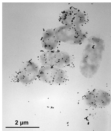
Figure 3.26 TEM image of fresh Bacteria@AgNPs sample.
