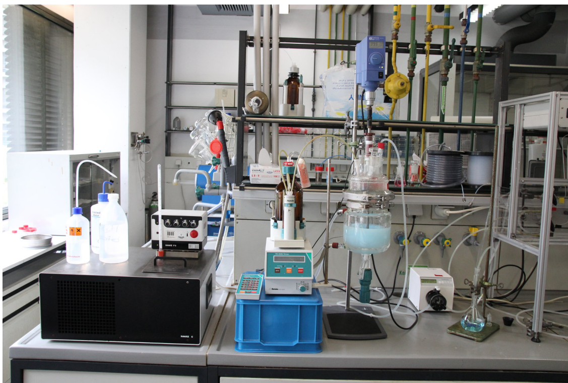
Figure 3.1: Experimental setup for the precipitation of copper catalysts.
