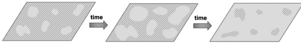
Scheme 2. Schematic representation of time-dependent gradual film formation, with coexistence of different stages of latex particle coalescence.
