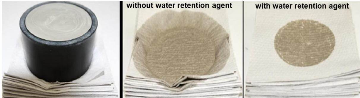
Figure 5: Illustration of the filter paper test used for quantification of the water retention of a plaster.
