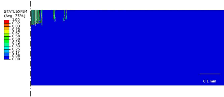
Figure 4.22: Cracks predicted by XFEM simulation for a thermal shock load of 0.5 \text{ GW/m}^2 .
