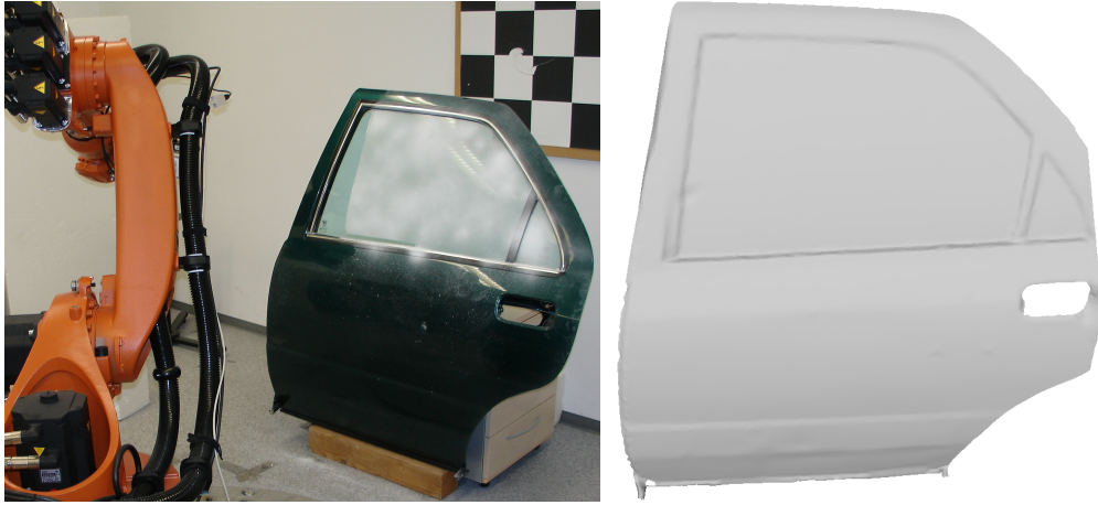
Figure 5.8: For a Lancia car door, NBS are iteratively planned utilizing the industrial robot (left) and resulting in a reasonable 3D triangle mesh (right).
