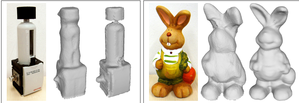
Figure 1.3: Comparison of the performance of KinectFusion with our autonomous modeling system on a pneumatic filter (left box) and a bunny (right box) object. In each box from left to right: picture of object, mesh generated with KinectFusion and mesh created with the autonomous modeling approach suggested in this thesis. For KinectFusion, the details in the objects are lost and also the object proportions are incorrect.
