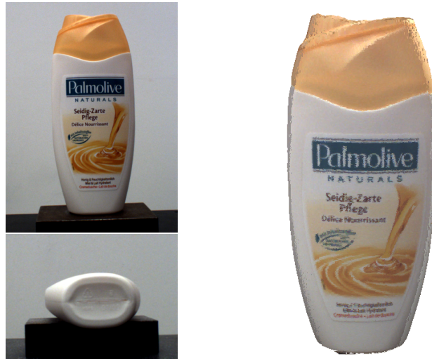
Figure 5.9: Autonomous object modeling of a shower gel including texture. Top left: Image from front mono camera view of object in initial position. Bottom left: Image from front view after moving object to the side. Right: Textured 3D Model.
