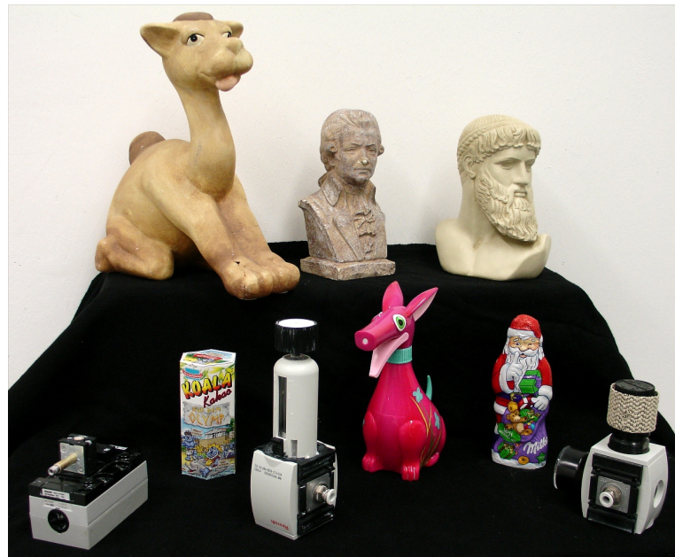
Figure 5.4: The objects used during the geometric modeling experiments. Top: camel, Mozart and Zeus (cultural heritage). Middle: cookies, dog spray and Santa Claus (household). Bottom: control valve, filter and pressure valve (industrial). The largest object is the camel with 340 mm height, the smallest the control valve of 95 mm.
