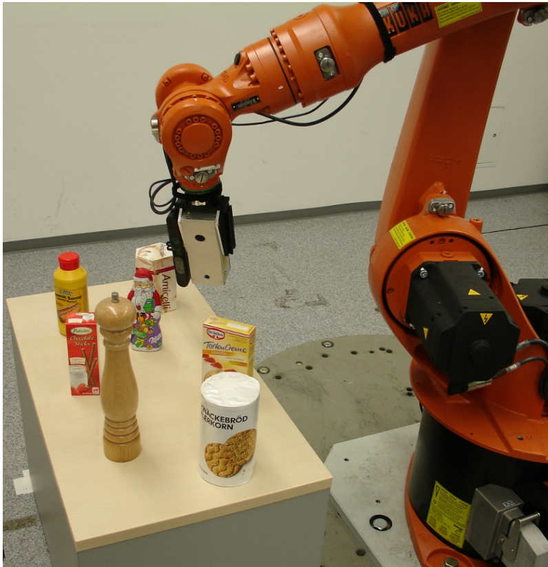
Figure 5.18: The setup for the industrial robot during active scene exploration: the objects are placed on a tabletop which allows for viewing the objects all around up to a certain distance. The stereo camera system has been removed as it makes the sensor head very bulky and restricts the possible sensor positions when moving into the initially unknown scene.
