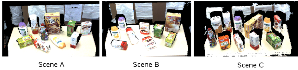
Figure 5.11: From left to right: range images with the stereo system of table top scene A, B and C. The scenes are used to evaluate the colored 3D models by pose estimation.
