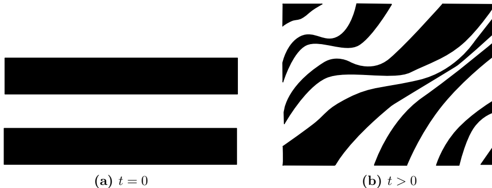
Figure 2.10: Illustration of fluid dynamic species mixing by turbulent convection [79]
