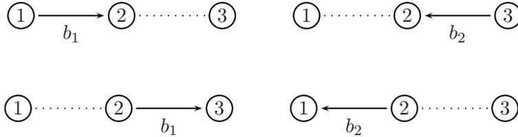
Figure 3.2: Two-way relaying in four steps (4P with DF, 0.5 bps / 2.0 lpb / 2.0 npb)
