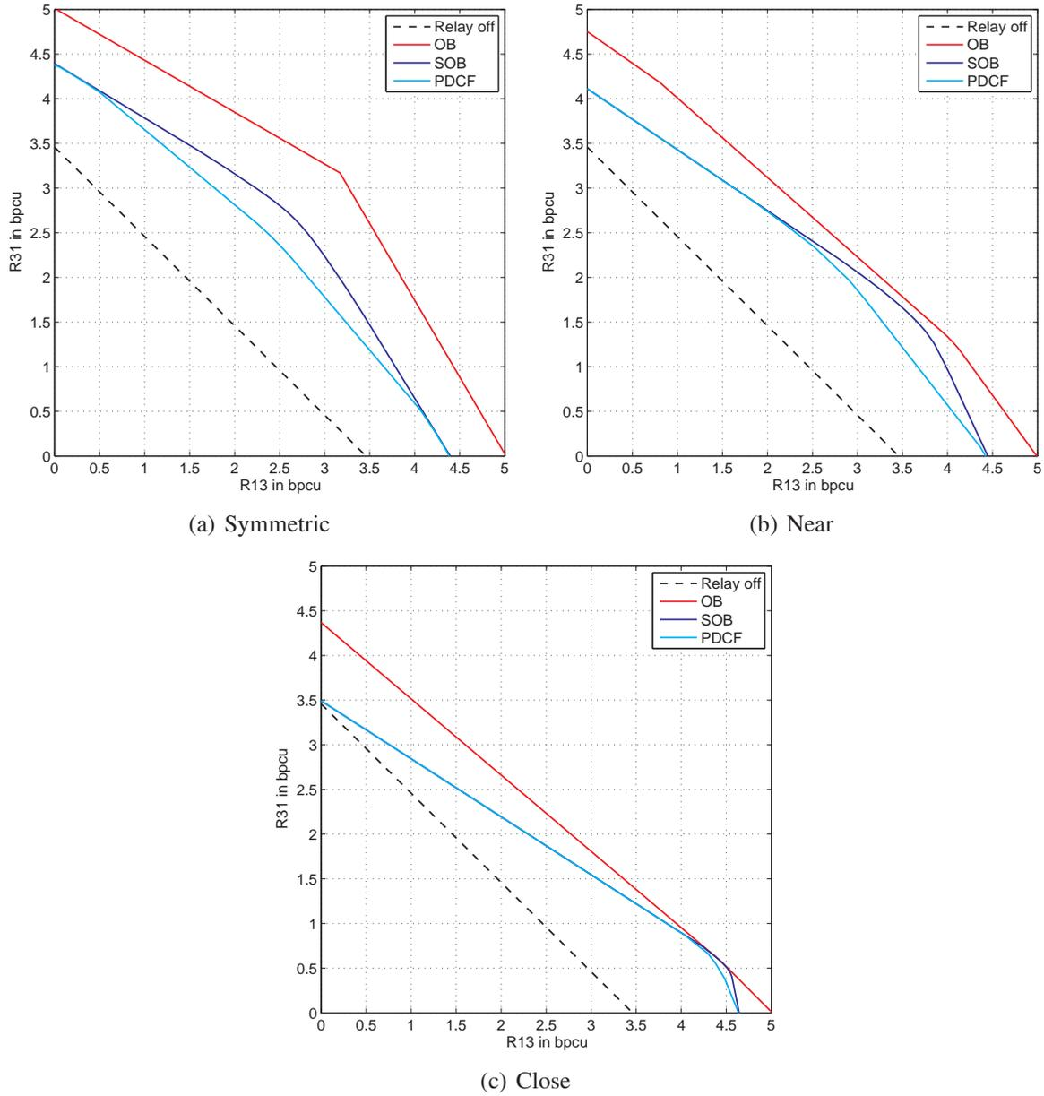
Figure 3.25: 3P-MA with PDCF, Line Network with  $P_i^{(l)} = 10$ ,  $\alpha = 3$
