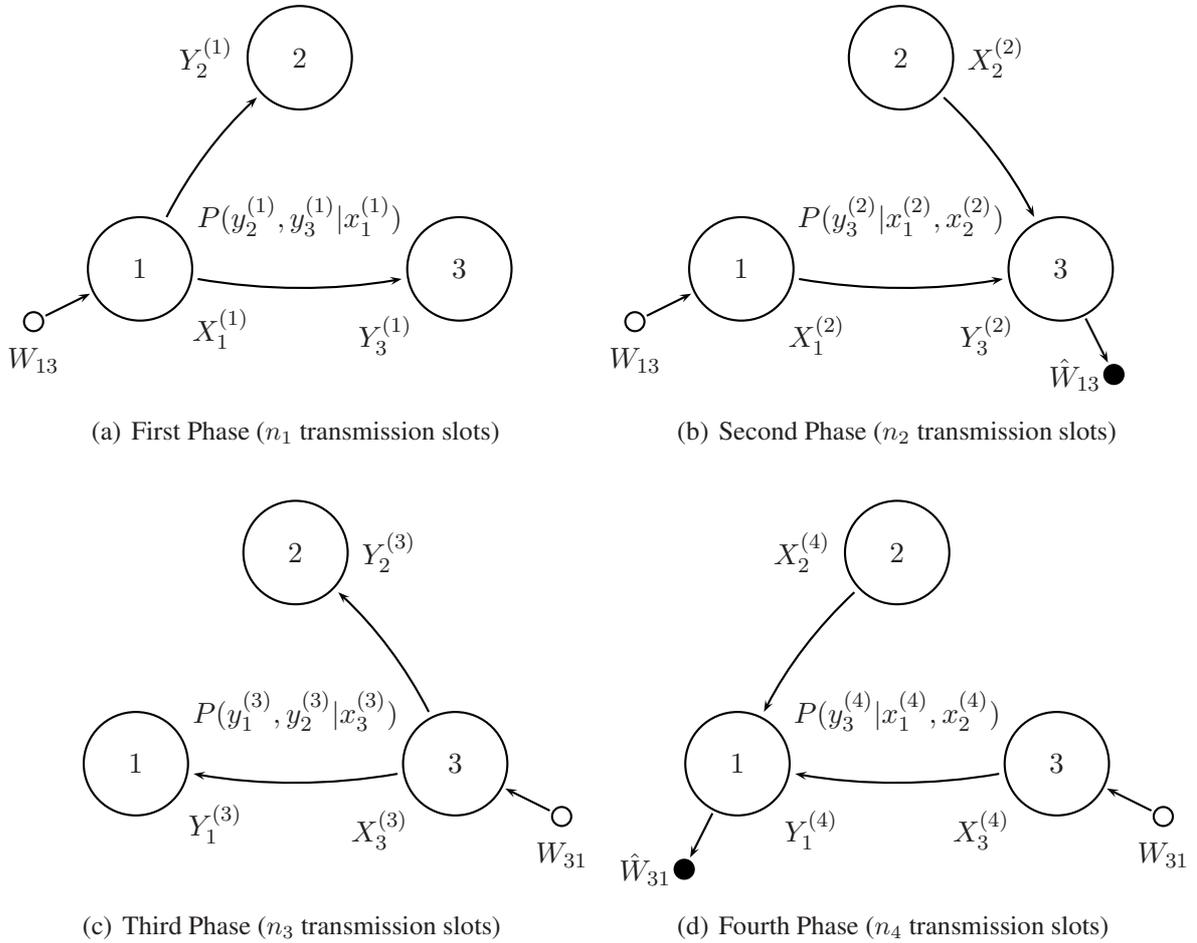
Figure 3.13: Half-Duplex Two-Way Relay Channel: 4P-OWRC Scheme
