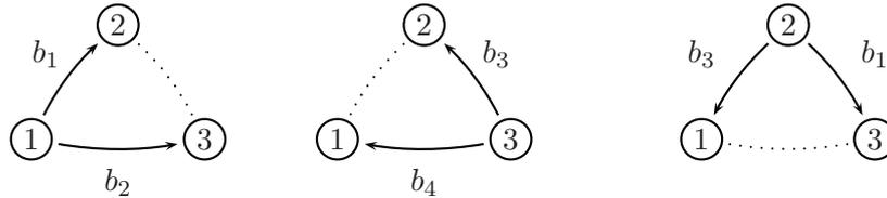
Figure 3.6: Two-way relaying in three steps (3P-BC with PDF, 1.33 bps / 1.5 lpb / 0.75 npb)
