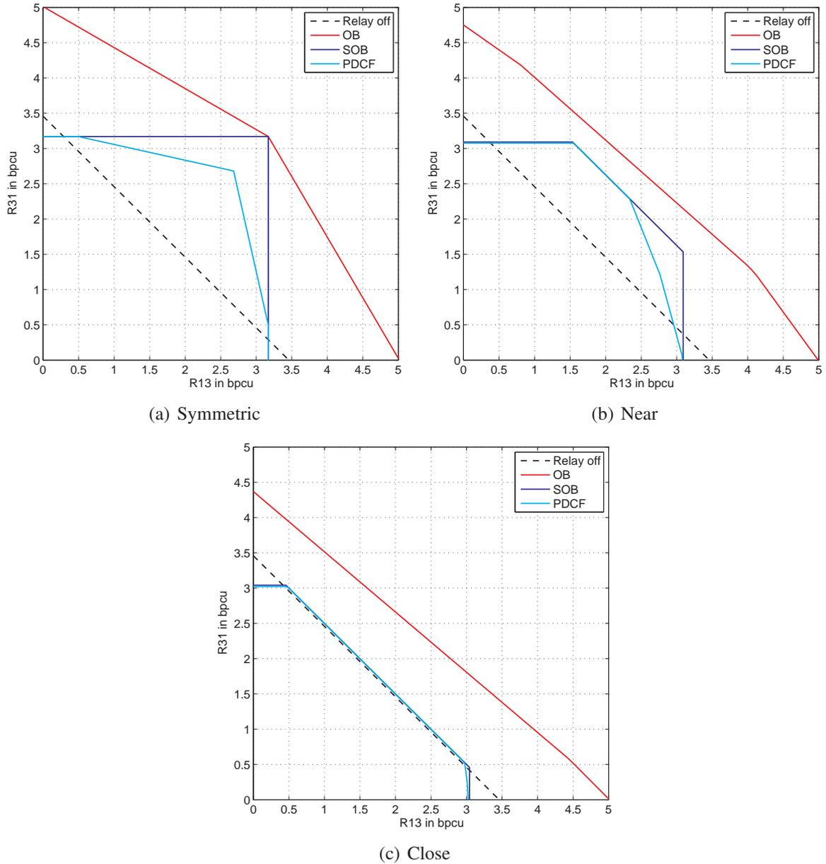
Figure 3.17: 2P-MA-BC with PDCF, Line Network with  $P_i^{(l)} = 10$ ,  $\alpha = 3$
