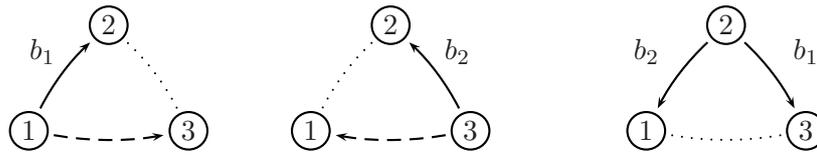
Figure 3.5: Two-way relaying in three steps (3P-BC with DF, 0.67 bps / 2.0 lpb / 1.5 npb)
