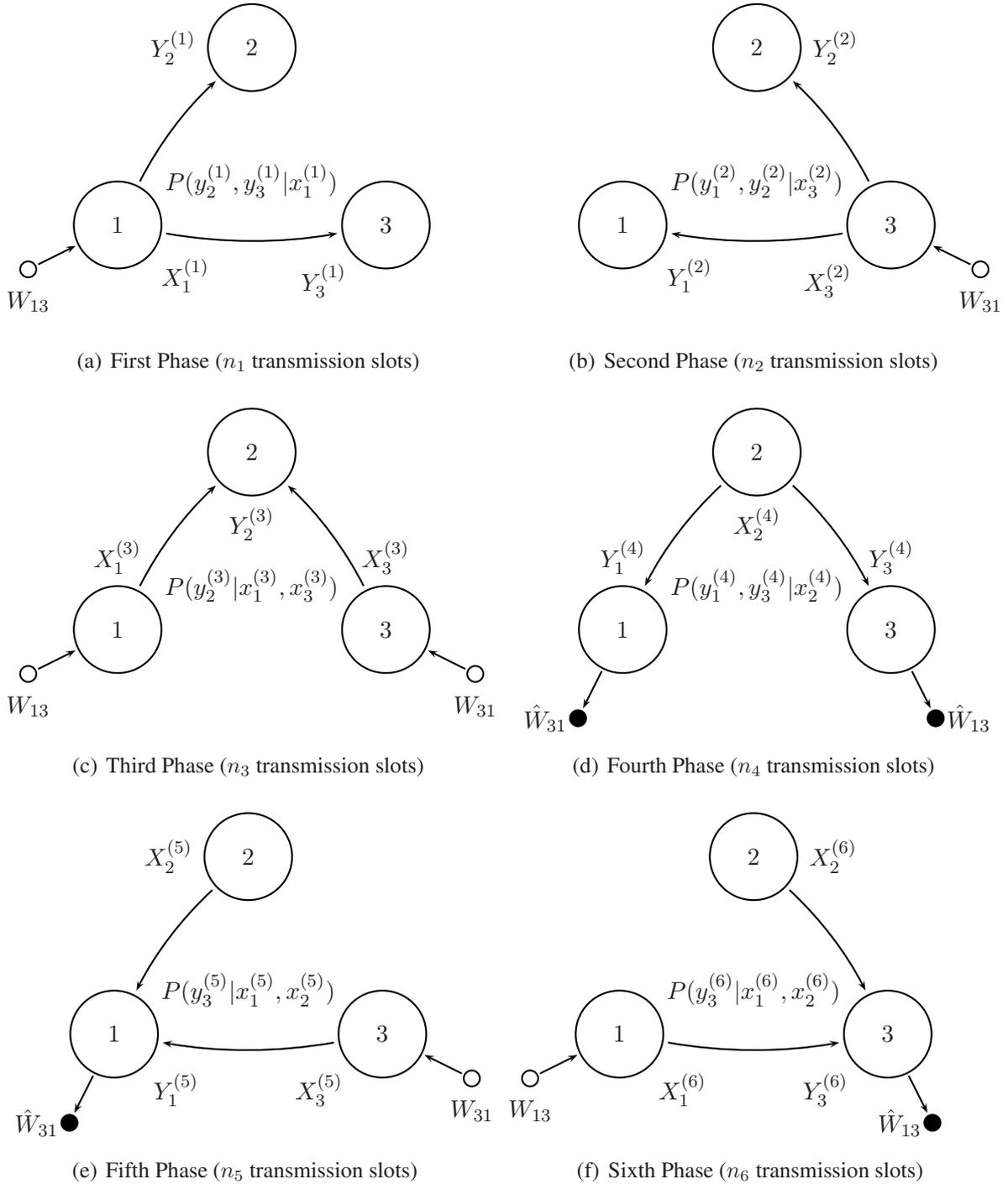
Figure 3.14: HD-TW Relay Channel: 6P Scheme
