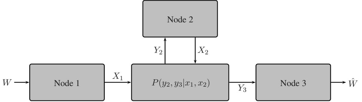
Figure 2.1: Full-Duplex Relay Channel
