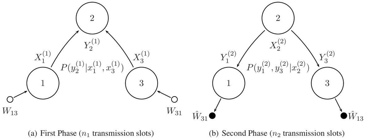
Figure 3.10: HD-TW Relay Channel: 2P-MA-BC Scheme
