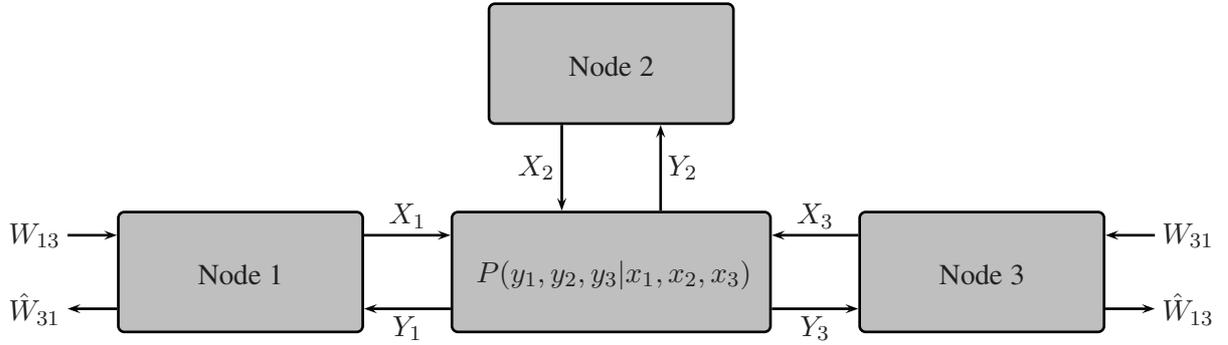
Figure 3.8: Full-Duplex Two-Way Relay Channel
