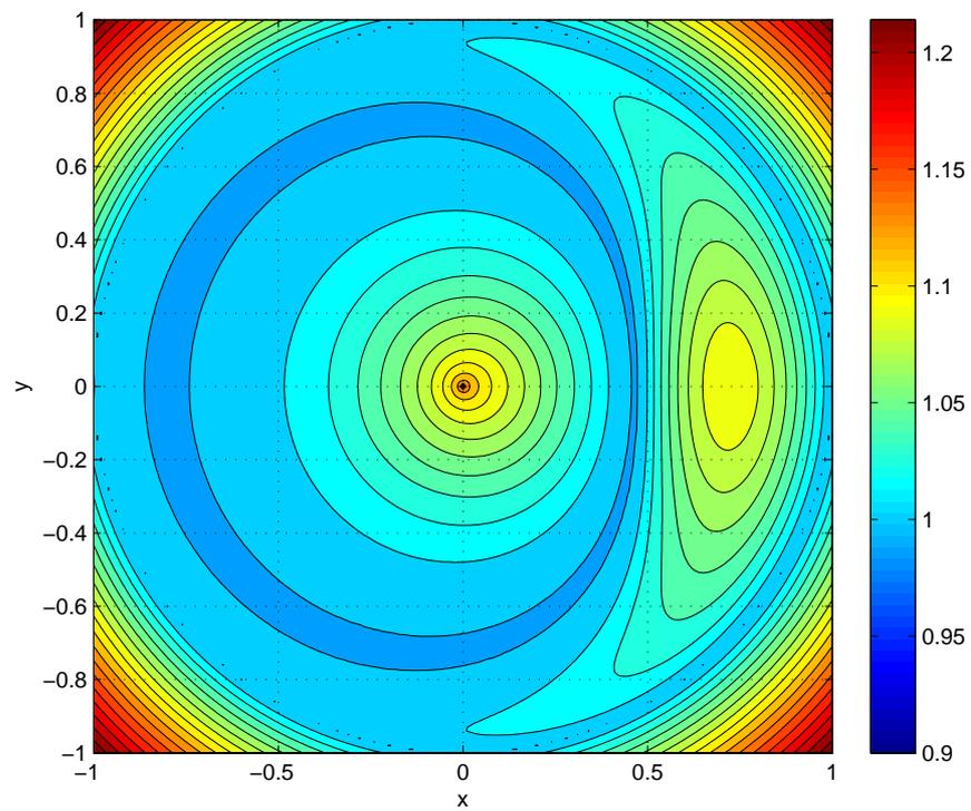
Figure 2.10: Rate Gain for DF with TA, Plane Network with  $P_i^{(l)} = 10$ ,  $\alpha = 3$
