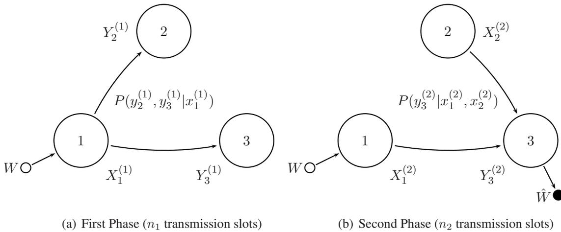
Figure 2.2: Half-Duplex Relay Channel
