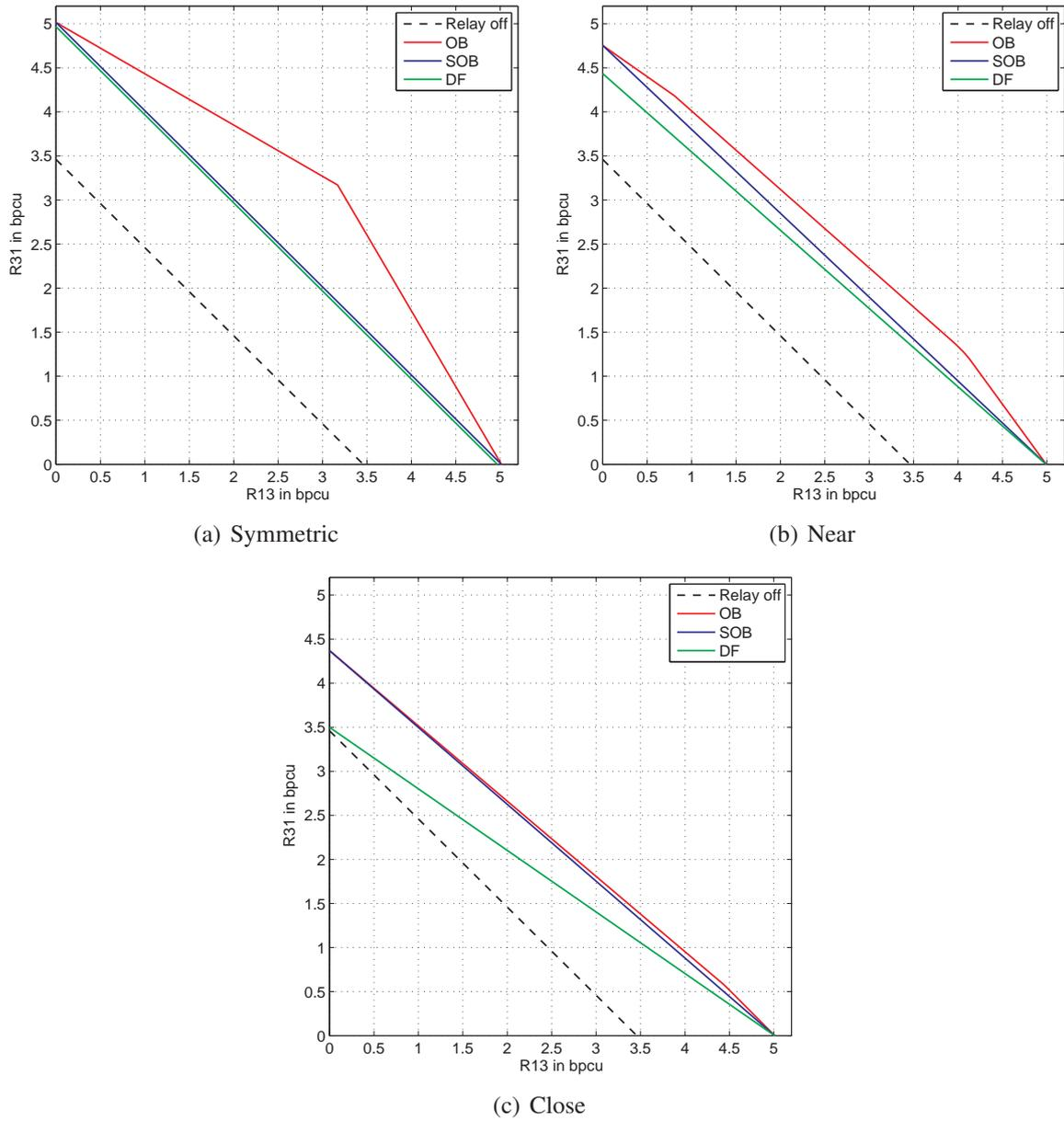
Figure 3.27: 4P-OWRC with DF, Line Network with  $P_i^{(l)} = 10$ ,  $\alpha = 3$
