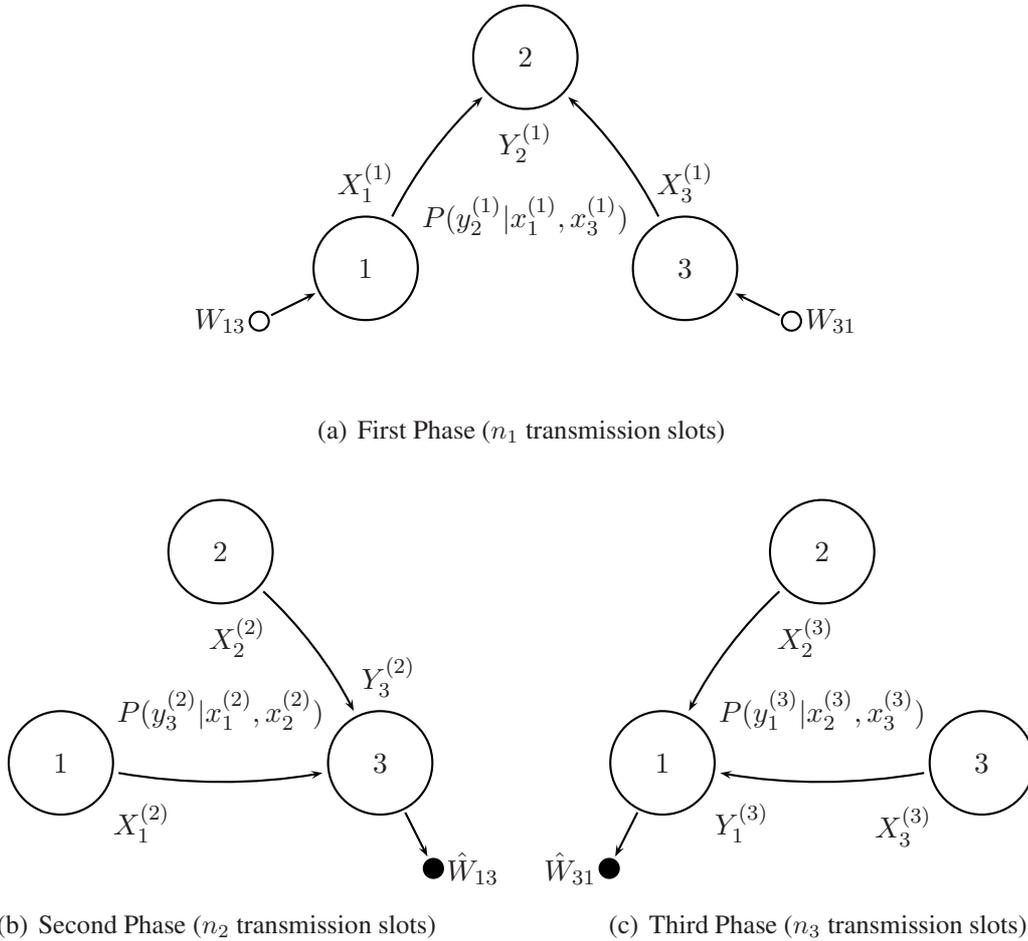
Figure 3.12: HD-TW Relay Channel: 3P-MA Scheme
