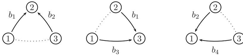
Figure 3.4: Two-way relaying in three steps (3P-MA with DF, 1.33 bps / 1.5 lpb / 1.5 npb)
