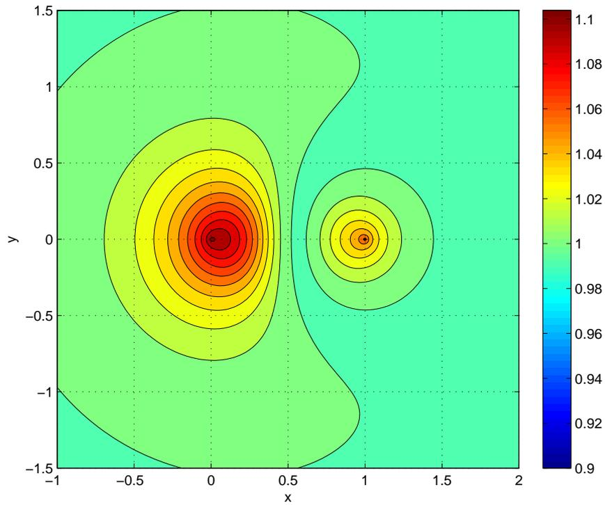
Figure 2.11: Rate Gain for CF with TA, Plane Network with  $P_i^{(l)} = 10$ ,  $\alpha = 3$
