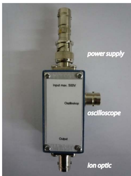
Figure 4.8: Home built capacitive decoupled device used to measure the time distribution of the cluster beam on every ion optic.
