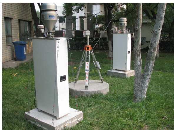
Figure 3.3: The location of the sampling site at the CUGB in Beijing from 21 June 2010 till 20 June 2011: sampler A and B as well as an ultra-sonic anemometer used to check the local transport conditions
