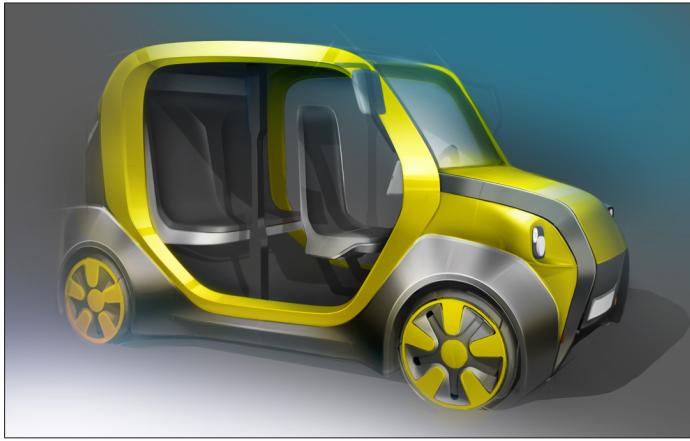
Figure 6. Design study of the multi-modal vehicle, which shows a version without doors. The design of the car is derived from the saint Bernard dog and shall indicate the helpful character of the vehicle. The interior is simple and well structured to enable an easy use for everybody. Just the absolutely necessary driving elements are realized within hardware - all other functionality is realized within software.
