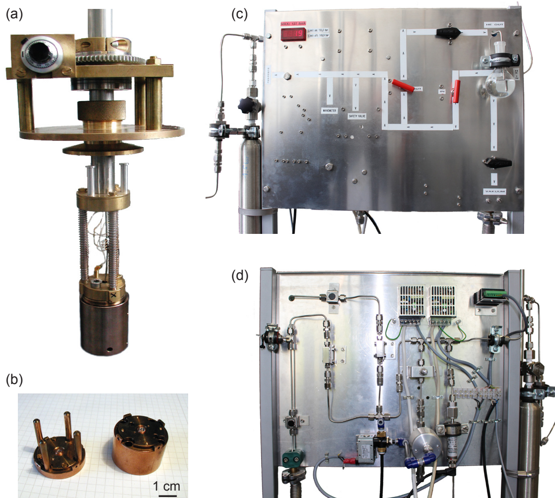
Figure 2.10: Photographs of the high pressure equipment built up during this dissertation. (a) dip stick with pressure cell, (b) open pressure cell, and (c, d) the gas handling system (front- and back-view) to adjust the applied pressure.
