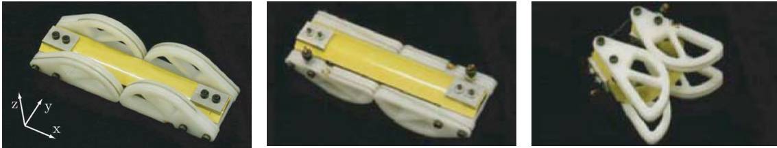
Abb. 41: TSR Hinge, Bimetall-Gelenk [82]
