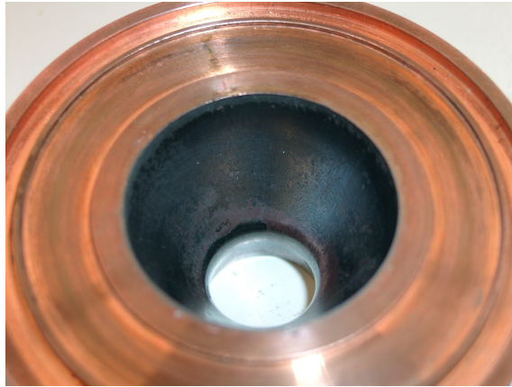
Fig. A.4: Detail of Nozzle Segment After Test (37 mm CC, \varepsilon_c = 5.0 )
