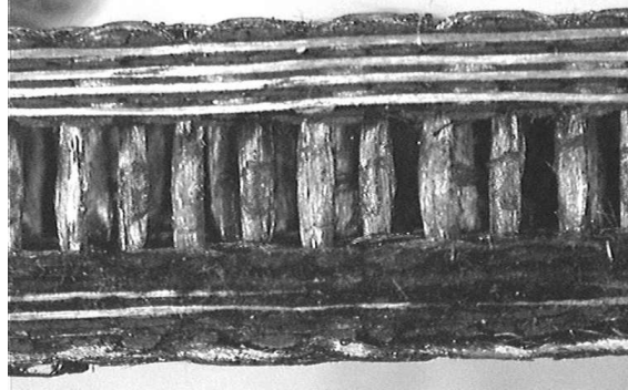
Fig. A.11: Detail of PTAH-SOCAR Duct with Fin Structure (Courtesy of MBDA France)
