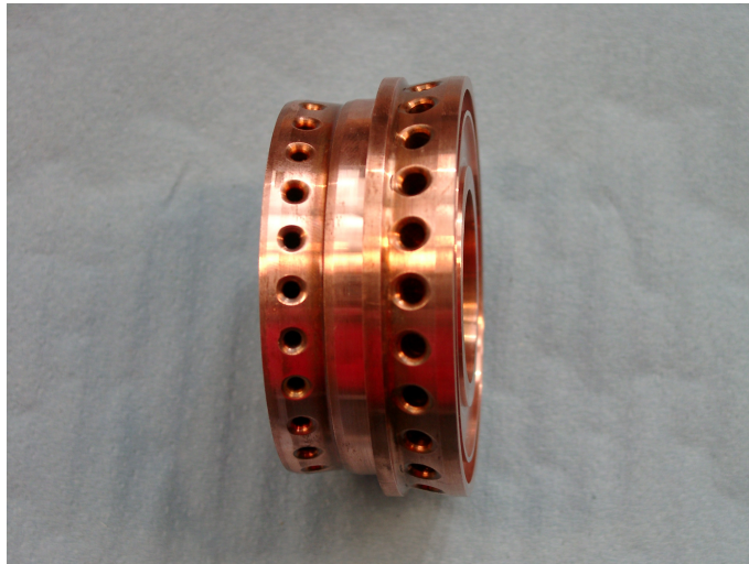
Fig. A.2: Water-Cooled Segment for 37 mm Combustion Chamber (with holes for hot wall temperature measurements)
