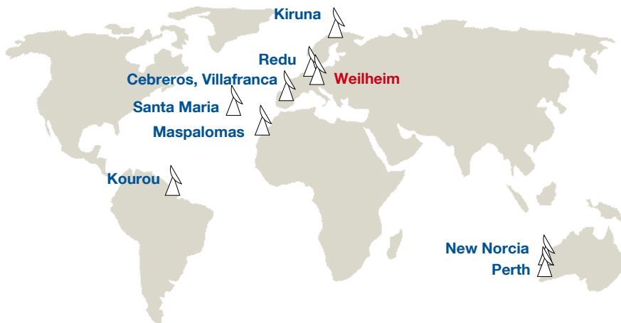
Figure 2.5: Sites of the core network of ESA's ESTRACK ground station network and location of the ground station Weilheim I.
