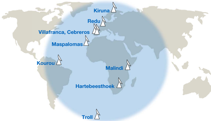
Figure 5.5: The blue area shows the maximum region a GEO satellite at 10^\circ longitude can cover on the ground. In addition, the visible ground stations of the ESA ESTRACK ground station network are marked.
