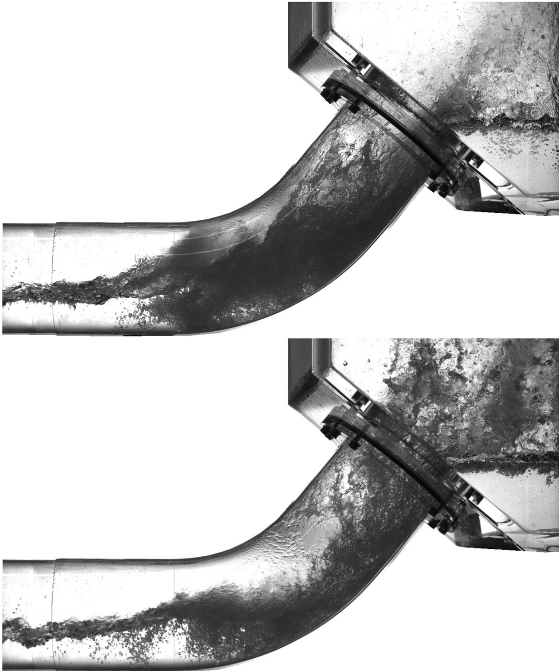
Figure 7.24 The air/water interface during the bend-CCFL. Upper image: A large roll-waves approaching the bend and blocking almost the entire cross section of the pipe. A strong annular churn flow occurs at the bend/riser region. Lower image: The remaining of the wave crest, droplets, and the foam after it crashes into the SGs. The intensity of the CCFL mechanism is remarkably higher as in the first region. J_w^{*0.5} = 0.155
