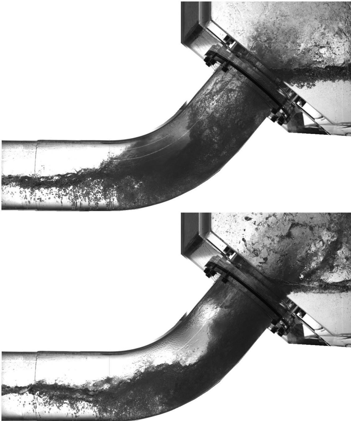
Figure 7.33 The air/water interface during the bend-CCFL. Upper image: A large roll-waves blocking the entire cross section of the pipe. An intense annular churn flow accompanied with a large amount of foam formation occurs at the bend/riser region. Lower Image: The remaining of the two-phase mixture after it is pushed into the SGs. The bend-CCFL mechanism remains the same, however the intensity and amount of water carried backwards is increasing J_w^{*0.5} = 0.255
