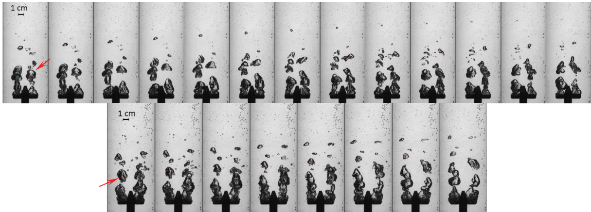
Figure 5.8 Snap shots for condensing steam bubbles from HIN32X0.8mm injection nozzle. Flow conditions: J_L = 0.2 \text{ m. s}^{-1} , T_L = 98^\circ \text{ C} , dt = 6.67 \times 10^{-3} \text{ s} up: J_S = 0.09 \text{ m. s}^{-1} , \Delta T_{\text{sub}} = 5.7^\circ \text{ K} , bottom: J_S = 0.22 \text{ m. s}^{-1} , \Delta T_{\text{sub}} = 5.6^\circ \text{ K}
