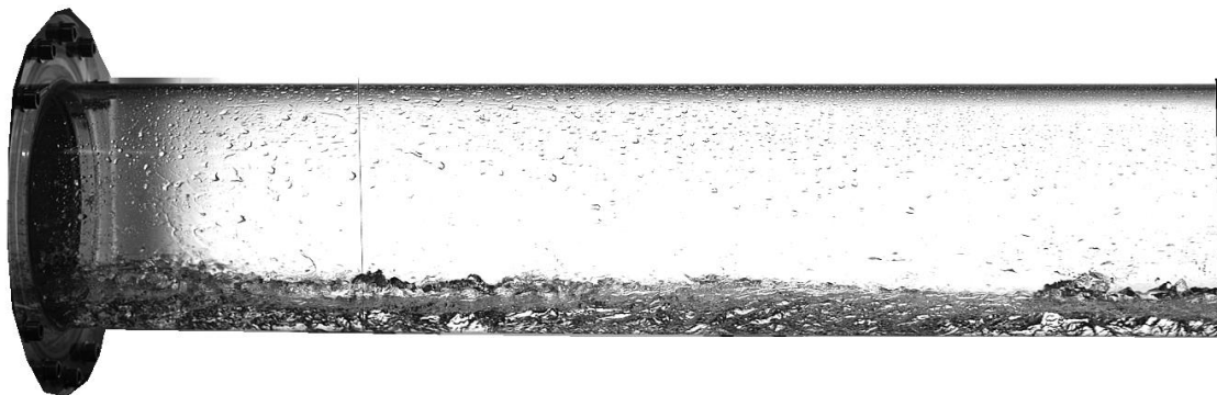
Figure 7.43 The air/water interface near the water exit during the onset of ADE-CCFL. The water stream surface is highly turbulent (though not subcritical), with a strong formation of droplets inside the entire horizontal section. J_w^{*0.5} = 0.305 .
