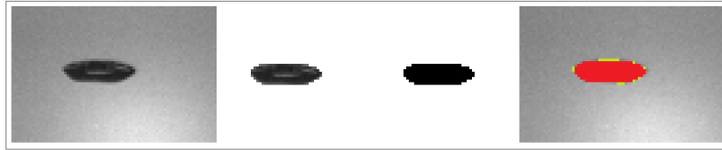
Figure 4.12 Illustration of the error made by the identification procedure. Left to right: Raw image, identified bubble's area, manually identified bubble, and superimposed images (green pixels represent those not counted by the procedure).
