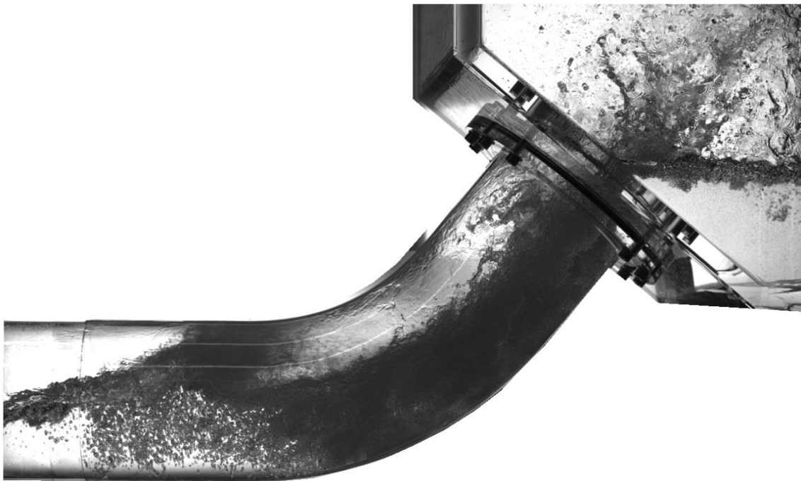
Figure 7.49 A large roll-waves that blocks the air flow during the Bend-CCFL. J_w^{*0.5} = 0.305 .
