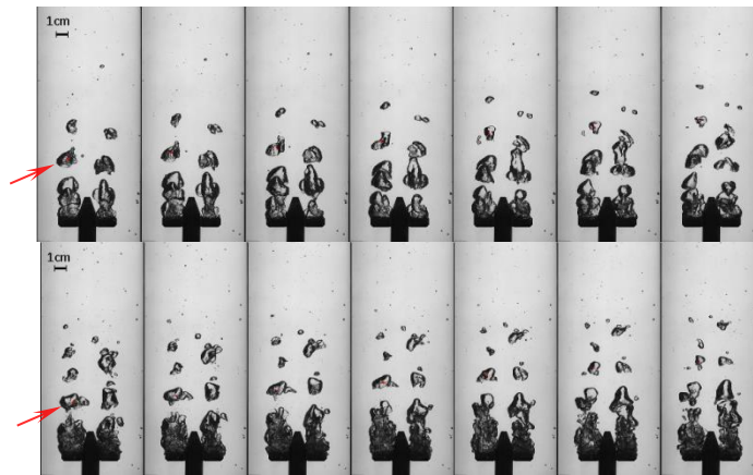
Figure 5.9 Snap shots for condensing steam bubbles from HIN32X0.8mm injection nozzle. Flow conditions: J_L = 0.4 \text{ m. s}^{-1} , T_L = 98^\circ \text{ C} , dt = 6.67 \times 10^{-3} \text{ s} up: J_S = 0.09 \text{ m. s}^{-1} , \Delta T_{\text{sub}} = 6.7^\circ \text{ K} , bottom: J_S = 0.22 \text{ m. s}^{-1} , \Delta T_{\text{sub}} = 6.2^\circ \text{ K}
