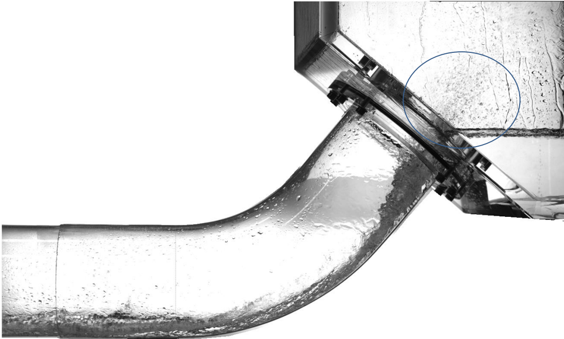
Figure 7.30 The air/water interface during ADE-CCFL at the bend. A jet of water droplets can be seen at the inlet, this jet transports water back into the SGs which forms the second mechanism of CCFL occurrence.. J_w^{*0.5} = 0.255
