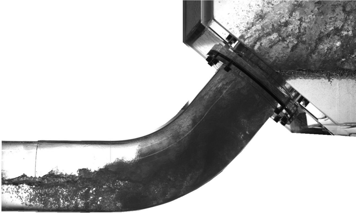
Figure 7.50 An intense, violent and turbulent annular churn flow during the Bend-CCFL. J_w^{*0.5} = 0.305 .
