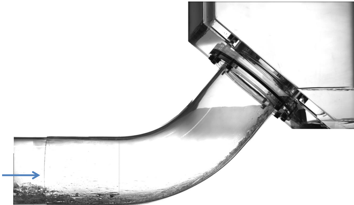
Figure 7.13 The approach of the hydraulic jump coming from the water exit towards the bend. J_w^{*0.5} = 0.105 .
