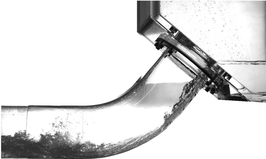
Figure 7.38 The air/water interface during deflooding. blower rotation speed (35%). Only a hydraulic jump remains at the bend with some droplets shedding off the surface. Eventually, the hydraulic jump moves towards the water exit transforming the flow back into a supercritical flow. J_w^{*0.5} = 0.255 .
