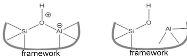
Figure 1.7: Illustration of nature of Brønsted acid sites (left) and Lewis acid sites (right) in zeolites (adapted from ref. 28 ).
