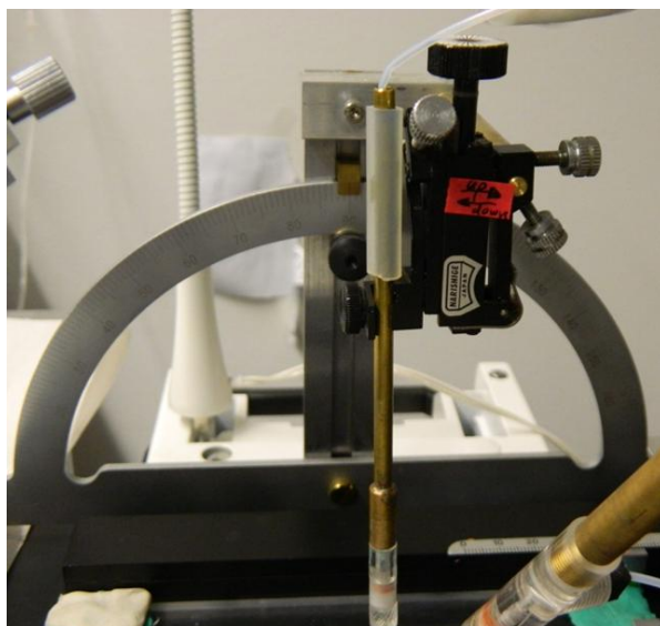
Figure 2.7: Custom-made arch for application of hydrostatic pressure with different angles used on the experimental set-up.
