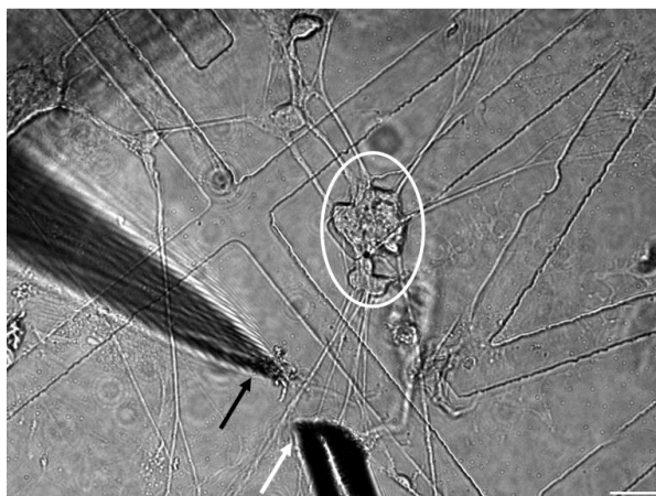
Figure 2.11: Picture of the experimental set for the local blockade of neuronal activity with tetrodotoxin (TTX). The neuronal cluster is encircled in white, the micropipette filled with 10 \mu\text{M} TTX is marked with a black arrow and the carbon fiber is marked with a white arrow. Scale bar: 20 \mu\text{m} .
