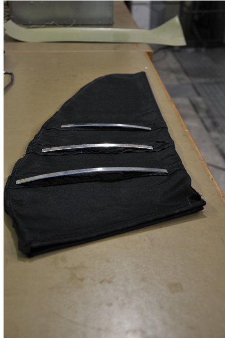
(b) Cambered battens to be fixed on the wing upper side
