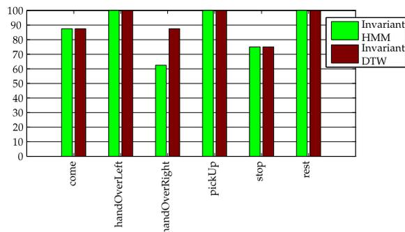
Fig. 6. The comparison between the recognition rates for the CM dataset.
