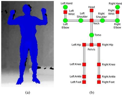
Fig. 2. (a) Human shape (blue) extracted from the depth map provided by the Kinect sensor. (b) Human skeleton model in which the circles and the squares represent the tracked human parts. Parts marked with the circles are effectively used in the Continuous Motion dataset of Sec. V-B.
