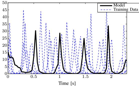
Fig. 4. Trained model (black solid line) of one of the invariant features obtained from five training demonstrations (blue dot-dashed lines).
