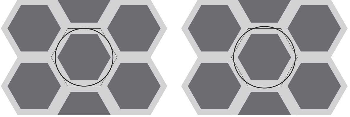
Figure 5.13: Illustration of the different simulation regimes (left: in-circle approximation, right: equivalent area approximation) used for the quasi-3-D device simulations.
