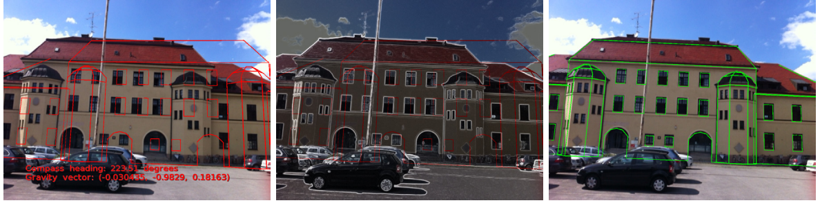
Figure 4.9: An edge model of the environment (left) together with the known ground truth camera position and the coarse camera orientation obtained from the attached sensors (center) enables recovering the ground truth orientation and therefore full 6DoF ground truth pose (right).
