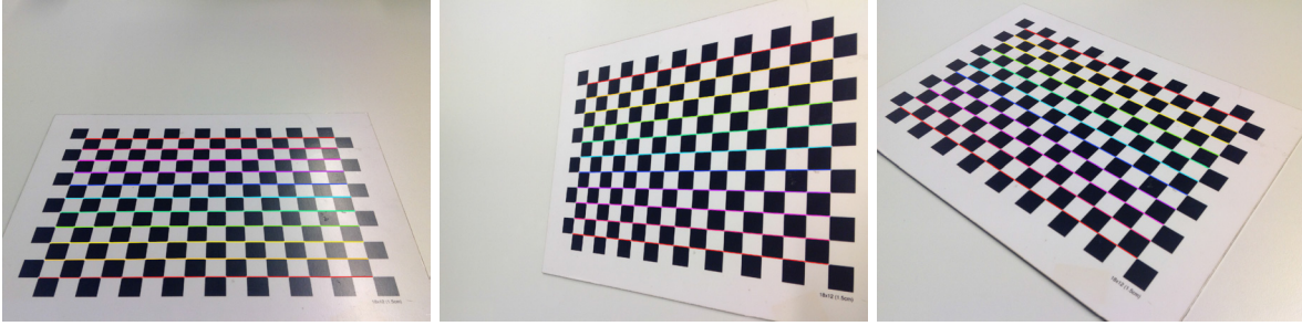
Figure 2.1: Three exemplary images used to calibrate the intrinsic parameters of a camera. The colored lines indicate that the checkerboard was successfully detected.
