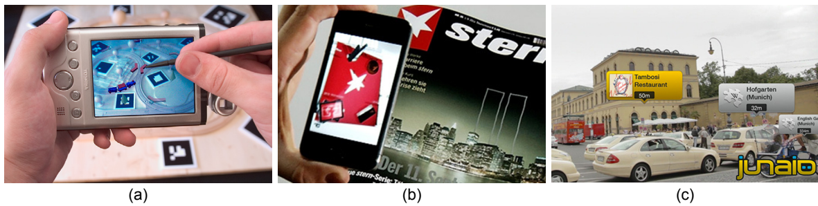
Figure 1.1: Examples for handheld Augmented Reality: Marker tracking (Courtesy of Vienna University of Technology) (a), planar object tracking (b) at the example of a magazine cover and non-visual tracking based on sensors (c) in junaio’s location-based channels.
