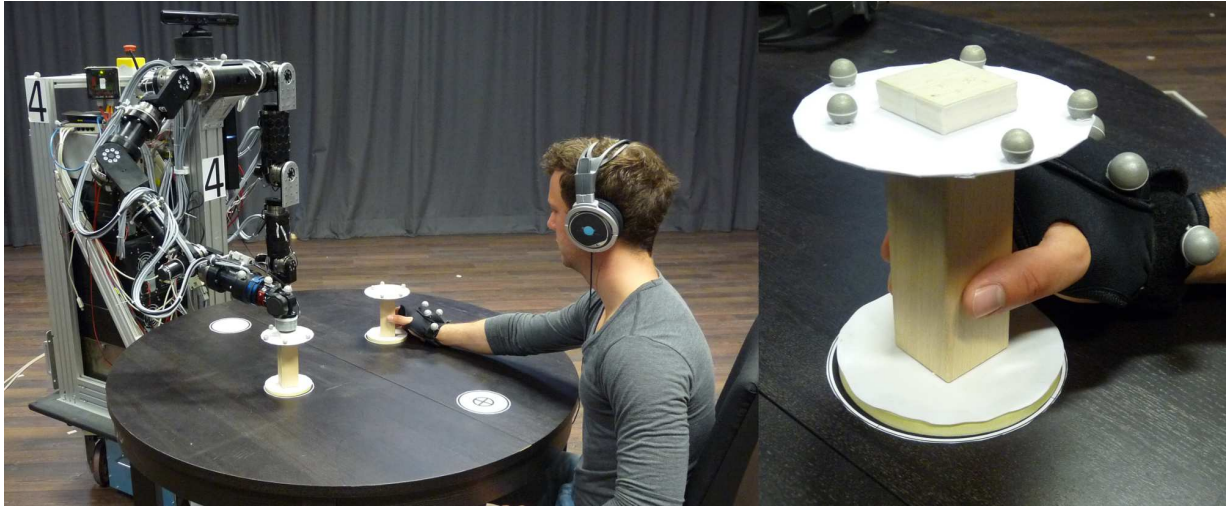
Fig. 4.15: The experimental setup and scenario of a prototypical joint pick and place task ( left ). Hand movements are made available to the robot in real time by tracking the glove the human interaction partner is wearing ( right ).
