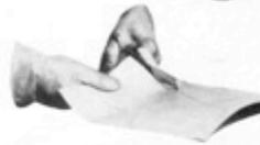
To cut templates a special scissors with double-edge blades is used. Distance of double edge equals thickness of the center wall of
