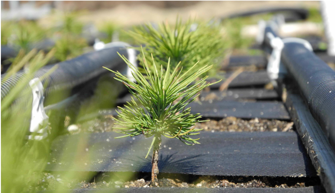
Figure 3.5 Seedling during heating period 2012 surrounded by black plastic tubes (mounted on top of wooden strips to prevent disproportionate soil heating) and the stripes of black water-permeable geomembrane
