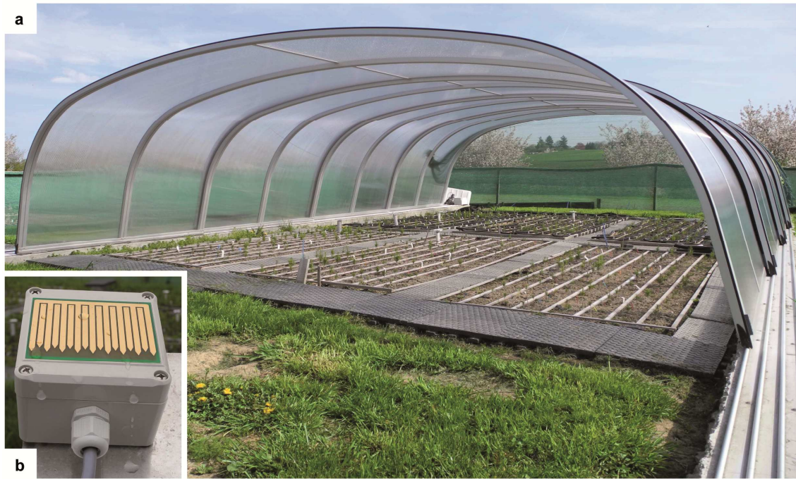
Figure 3.3 Installation for manipulation of precipitation with a) the rain-out shelter covering the dry and warm+dry treatment plots and b) the rain sensor that closes the rain-out shelter in case of rain
