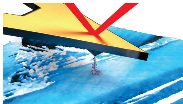
Figure 10. Schematic of an atomic force microscope cantilever with a laser reflected from the backside. The cantilevers used for single molecule force spectroscopy are around 200-300 \mu\text{m} in length and 20 \mu\text{m} in width with a tip height of 2.5-8 \mu\text{m} . A poly-L-lysine chain (several 100nm) is attached to the tip via a poly(ethylene) glycol linker (approximately 30nm).
