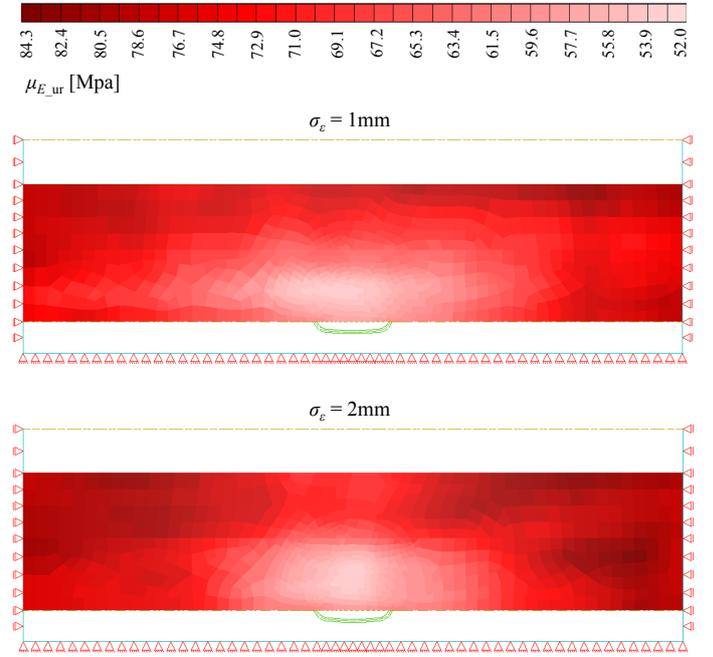
Figure 5: Posterior mean of the elastic stiffness modulus  $E_{\text{ur}}$  of the Keuper marl layer.
