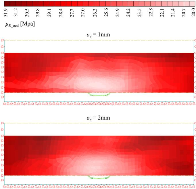
Figure 4: Posterior mean of the oedometric stiffness modulus  $E_{\text{oe}}$  of the Keuper marl layer.
