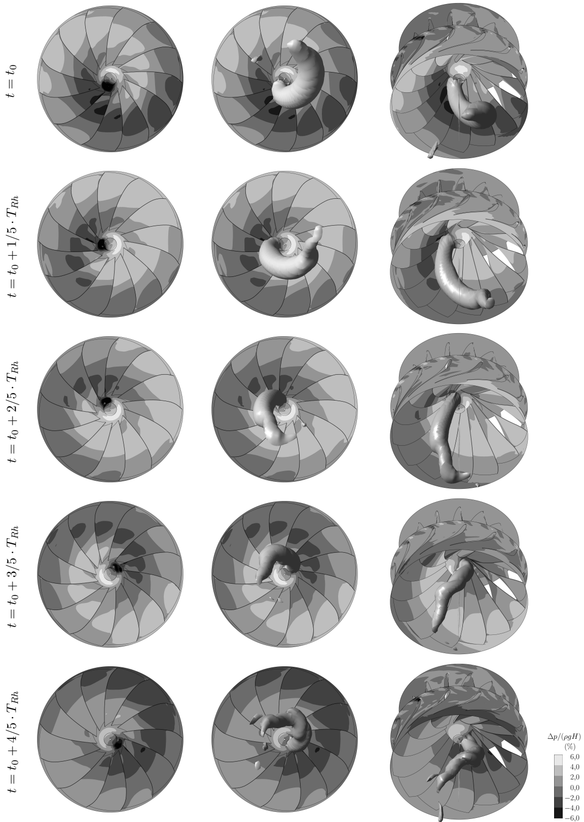
Figure 7.23: Pressure oscillations over one vortex rope rotation period at part load and high head viewed from the draft tube.
