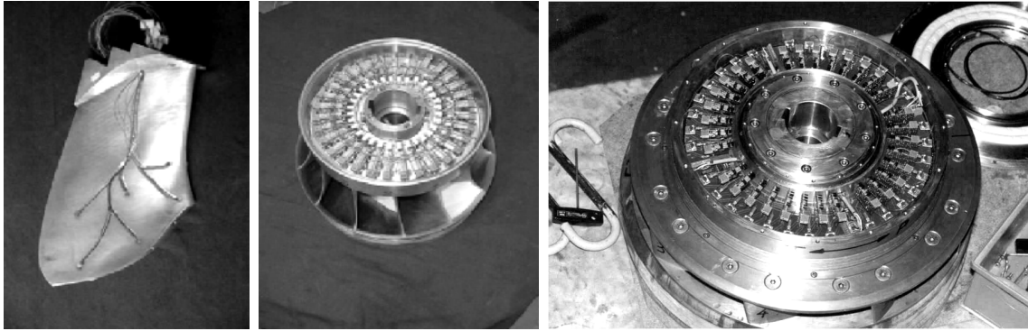
Figure 1.2: Typical experimental arrangement for measuring the pressure oscillations in Francis model runners. Pressure transducers at the blade (left) and acquisition equipment on the crown (centre, right). Reproduced from AVELLAN ET AL. [12].
