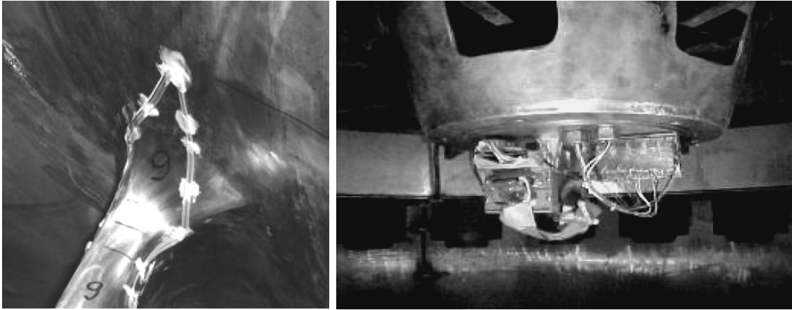
Figure 1.3: Typical experimental arrangement for measuring the pressure oscillations in Francis prototype runners. Strain-gauges at the blade trailing edge near to crown (left). Acquisition system mounted under the runner cone (right). Reproduced from FISCHER ET AL. [44].
