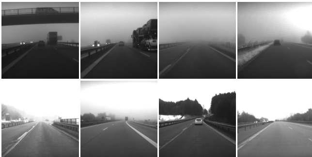
Fig. 7. Exemplary classification results. From top left to bottom right: The first two images show examples were falsely due to passing a bridge respectively overtaking a truck clear weather situations were detected (false negatives). The next two images show examples where our method has almost always detected fog situations correctly (true positives), this was e.g. the case for free road or for subsequent drives. The first two images of the second row show examples where fog was falsely detected (false positives). This occurred spontaneously and mostly in low-fog labeled images. The last two images show scenes correctly recognized as clear weather conditions (true negatives), one with basically high and one with basically low contrast, were both were trained with the same sample set.
