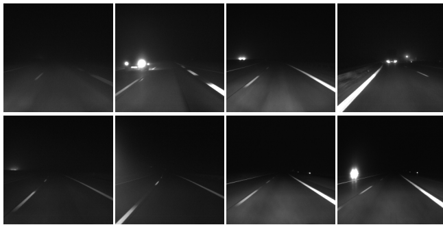
Fig. 8. Exemplary classification results for night-time scenes. From top left to bottom right: Each two examples of correctly detected fog scenes, falsely detected as fog-free scenes, falsely detected as fog scenes and correctly detected as fog-free scenes.
