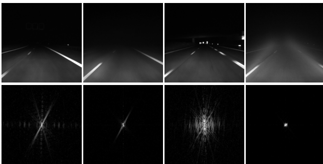
Fig. 5. Examples for clear and fog scenes at night. The top row shows the camera images the bottom row the corresponding power spectra. From left to right: No fog, fog, no fog and high beam, fog and high beam.
