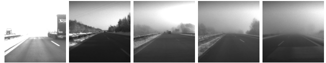
Fig. 6. Example images for labeling categories. Form left to right: Excluded, No Fog, Low Fog, Fog and Dense Fog.
