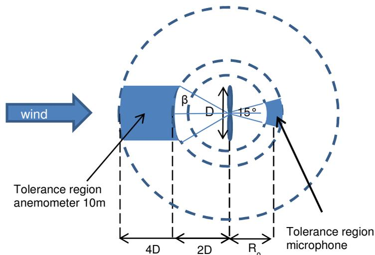
**Figure 1:** Top view of the basic measurement setup in accordance to IEC 64100. The possible locations for microphone and anemometer are indicated in blue.
