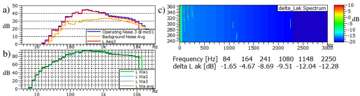
**Figure 3** a) Shows 3<sup>rd</sup> octave levels for operating and background noise and the resulting correction L Leq b) Sound powers of all three required time stamps and the resulting average c) The tonality as spectrum over time for two minutes, averaged tones are illustrated in the table below.
