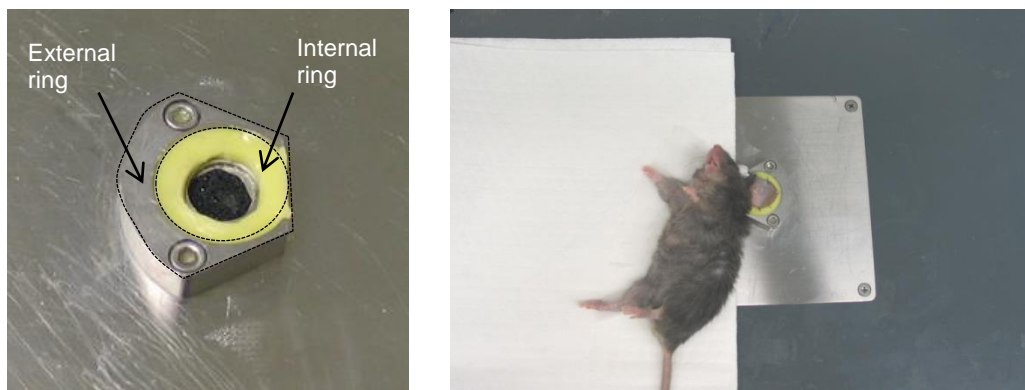
Figure 11. Stage for intravital microscopy in the mouse ear
