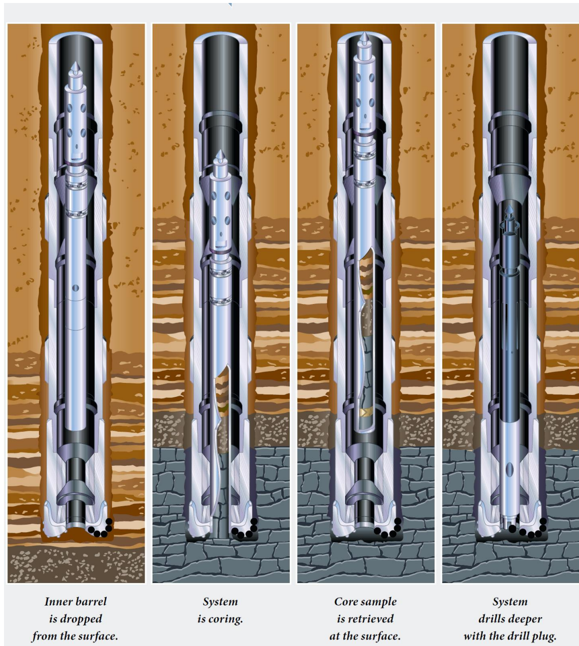
Figure 18: Schematic of a drilling plug allowing simultaneous drilling and coring (from [196])
