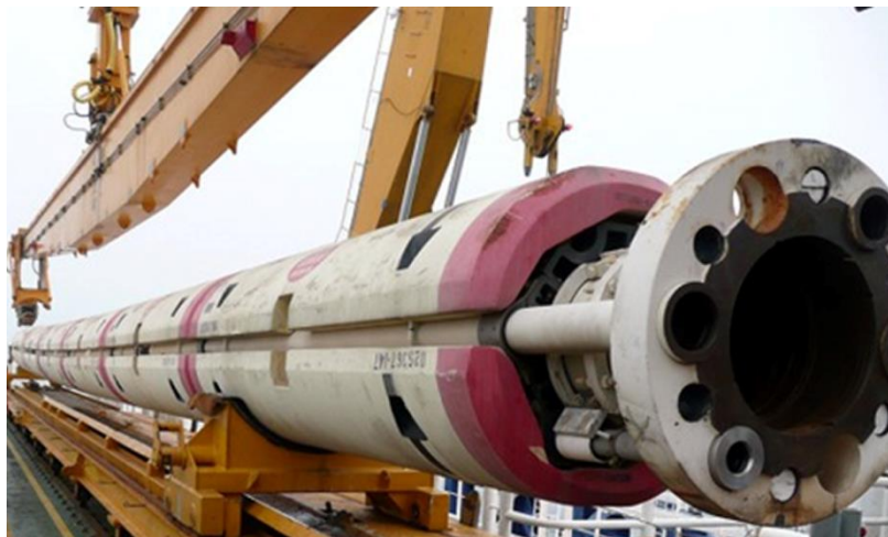
Figure 16: Riser for deepwater drilling [175]
