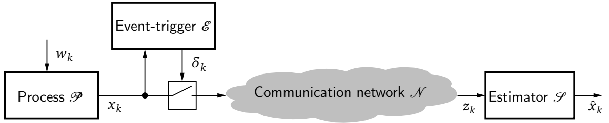
Figure 3.1: System model of the networked estimation system with plant \mathcal{P} , event-trigger \mathcal{E} , state estimator \mathcal{S} and communication channel \mathcal{N} .
