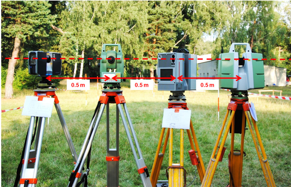
Figure 11: Instrument setup at TLS testing track
