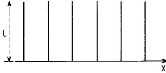
Figure 2.5: Diffusion on a comb-like structure [82]. The particle diffusion is normal, i.e. Brownian, along all sections of the comb. The motion in the x -direction is paused whenever the particle enters one of the spikes. If the spikes extend indefinitely, L = \infty , the mean time spent in a spike is infinite, so that the motion along the x -axis is a CTRW.
