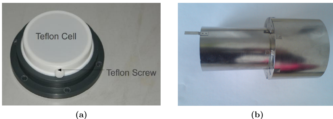
Figure 4.3: PTFE LS cell (a) and permalloy (b). Both have been customized in the workshop to meet the dimensions of the photo multiplier. Teflon has been chosen for the cell as it is inert towards liquid scintillators and features a high reflectivity around 430 nm. The mu metal was installed to compensate for magnetic fields.
