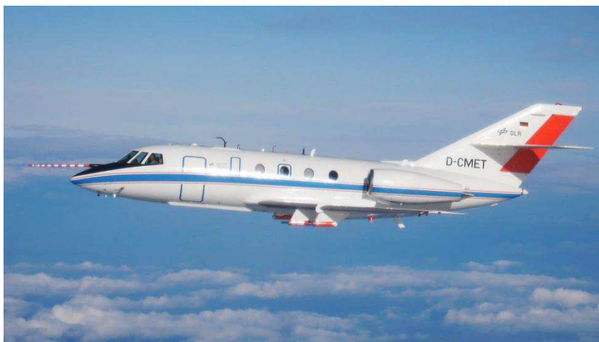
Figure 17. DLR research aircraft Falcon 20-E5 (D-CMET), hereafter referred to as Falcon. On the top the bent black aerosol inlet and below the wings the red cylindrical containers for the wing-mounted instruments are visible (source: http://www.dlr.de ).
