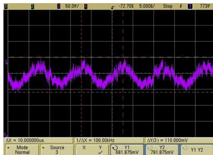
Figure 2.10: Disparity-generated sinusoidal tone with a frequency of 100 kHz at optical level of -28.5 dBm, additionally low pass filtered
