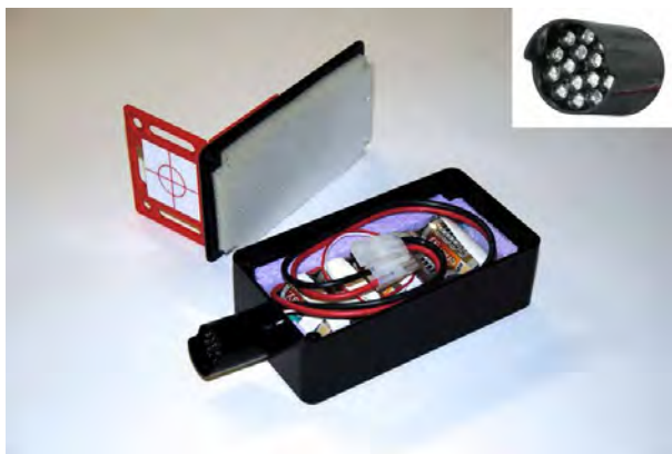
Fig. 2 | LED target in self-made isolated housing. Detail of LED cluster top right
