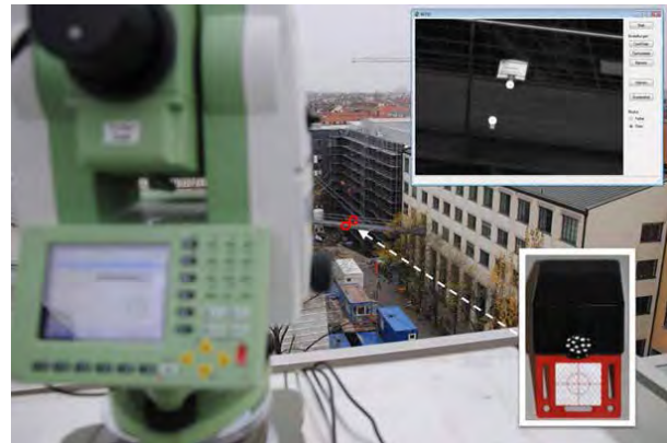
Fig. 3 | Test measurement at TUM campus with screenshot (top right) and used LED target (bottom right)
