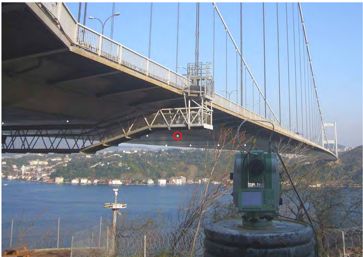
Fig. 6 | Fatih Sultan Mehmet Bridge seen from observation pillar with highlighted LED targets. The red circle indicates the IATS observed target.
