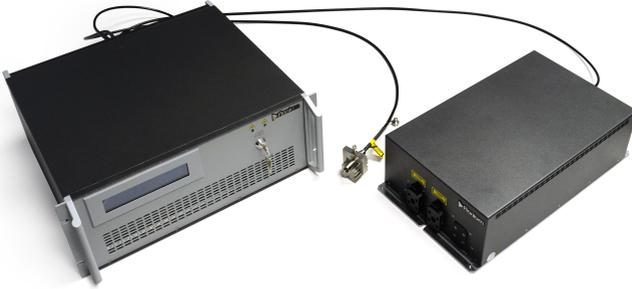
**Fig. 3.3 ALP laser source:** The system consists of three parts: A rack chassis (left) contains an infrared fibre master oscillator and super-continuum amplifier. A photonic crystal fibre guides light to a free-space collimator (center) for super-continuum output. More electronic and optical cables connect the chassis with the remote head (right). Here, amplification and spectral tailoring takes place for the two STED outputs. Image courtesy of Fianium Ltd.
