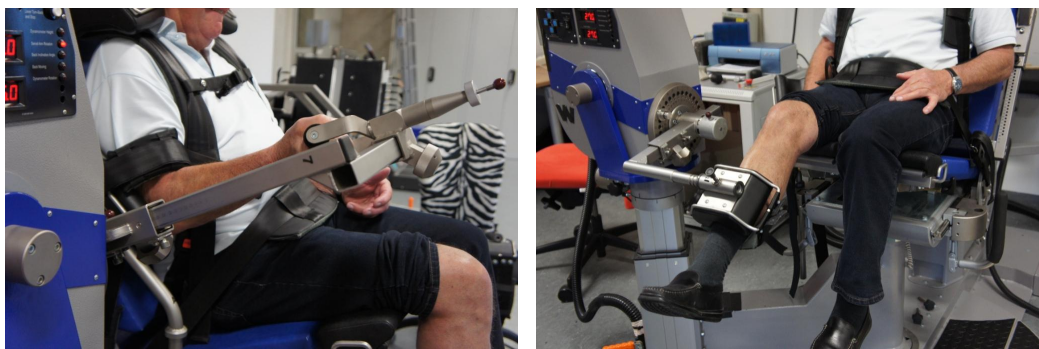
(a) Isomed setup for measurement of peak isometric elbow torque flexion (b) Isomed setup for measurement of peak isometric knee torque extension
